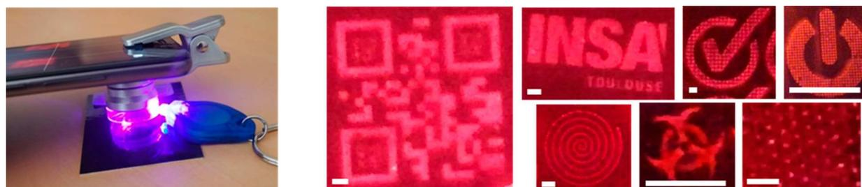
**Figure 5.** Reading of various PL tags using a smartphone equipped with a 20 $\times$  clip lens. Scale bars are 100  $\mu$ m.
