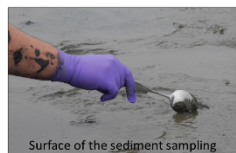
Surface of the sediment sampling Sieving at 100µm Picking of living specimens
