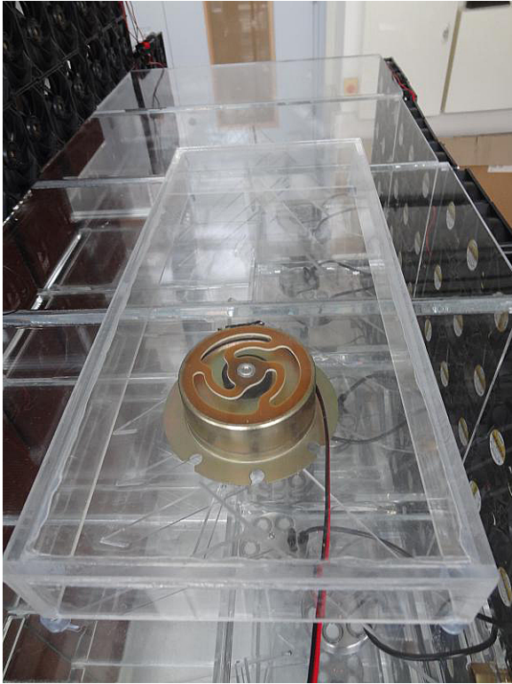
Figure 65. Vibrational Mighty Dwarf speaker positioned on top of the machine, behind the 4 units used for airflow. © Daniel Schorno, 2017.
