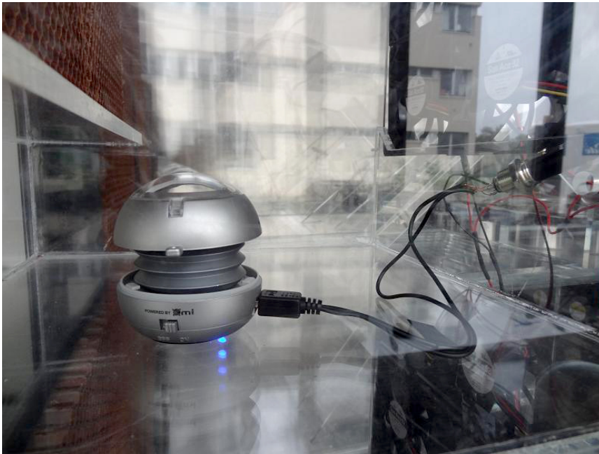
Figure 64. Xmini capsule speaker inside the dry unit of the cloud machine. © Daniel Schorno, 2017.
