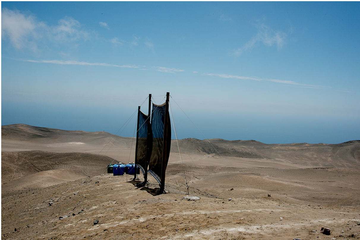
Figure 3. Two LFCs (Large Fog Collectors) with water tanks at the Alto Patache scientific site in Chile, south the city of Iquique. © Ana Rewakowicz, 2018.
