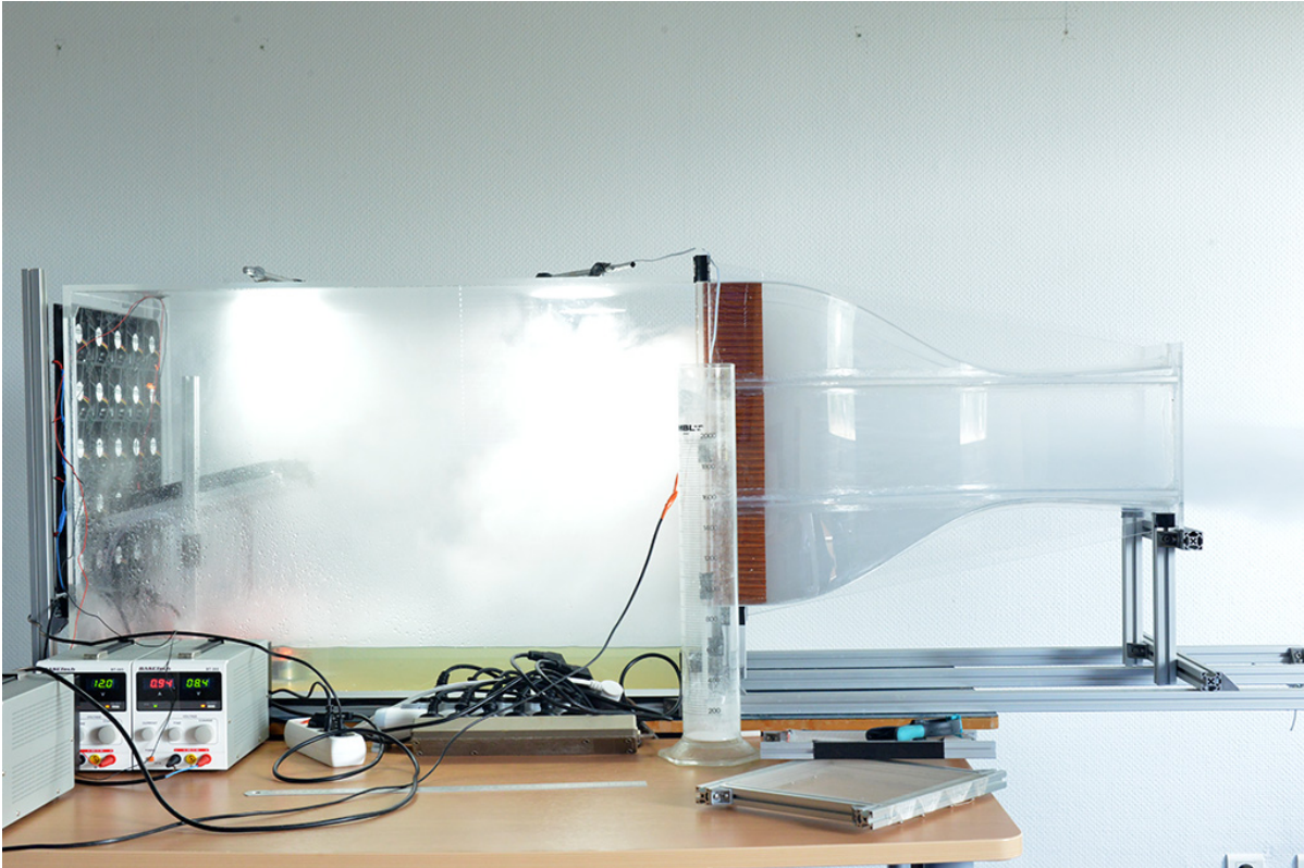
Figure 32. Wind tunnel fabricated by Romain Labbé to produce controllable fog. Ultrasonic foggers (not visible behind power supplies on the left) are covered with 1.5 cm of water. The first set of fans positioned almost horizontally above the foggers (middle-left) controls the amount of accumulated turbulent mass inside the middle chamber. The second vertical set of fans, seen on the left (black), controls the speed of the exiting fog, which is pushed through the honeycomb filter (brown, central) making the fog more uniform as it exits through the funnel (right). Both, fog's volume and speed are controlled by voltage adjustments on two power supplies operating two sets of fans separately. © Ana Rewakowicz, 2015.
