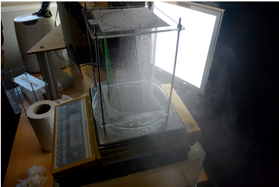
Figure 47. Hyperboloid presented in an experimental set-up, is another example of a ruled surface structure tested in collecting water from fog. Made with threads of different colours by students as part of the Architecting Water Collection summer course (École Polytechnique, 2015). © Ana Rewakowicz, 2015.
