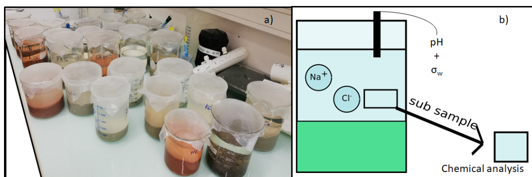
Figure 2.18: Monitoring of pH and water conductivity: a) Samples in which I monitored the pH and water conductivity, and b) diagram of the procedure.
