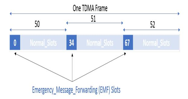
Figure 7.2: AS-DTMAC Multihop Frame.
