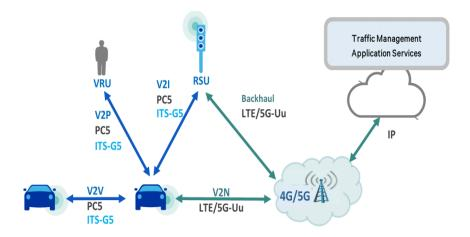
Figure 2.2: Hybrid architecture of a VANET with the relevant use cases (taken from the German project ConVeX:Deliverable D3.1)
