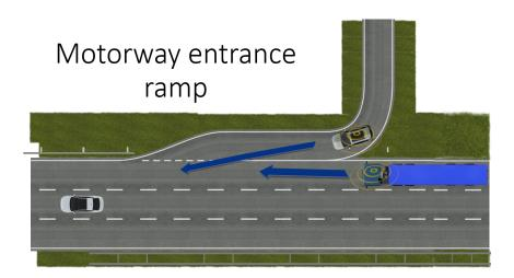
Figure 2.4: Motorway entrance assistance by using MCM messages.
