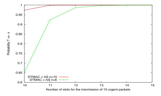
Figure 4.15: Cumulative distribution function of the number of slots required for the 10 urgent packets.
