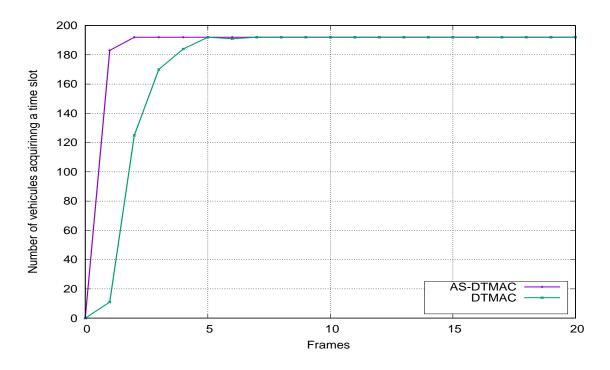
Figure 4.10: Number of vehicles acquiring a time slot within N frames.
