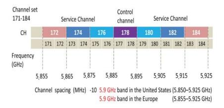
Figure 2.9: ITS-G5 spectrum band and channels in Europe & USA
