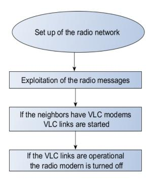
Figure 9.2: Algorithm to switch from the radio to the VLC link
