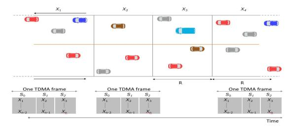
Figure 4.1: TDMA slots scheduling principle.
