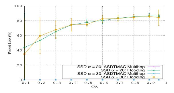
Figure 7.7: Packet Loss versus channel occupancy for AS-DTMAC Multi-hop and Flooding with error bar (95% confidence interval).
