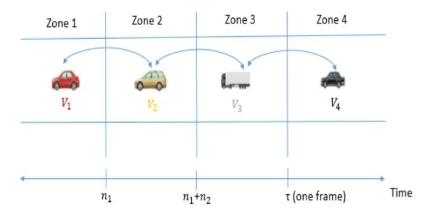
Figure 7.12: Message propagation based on TDMA slot information.
