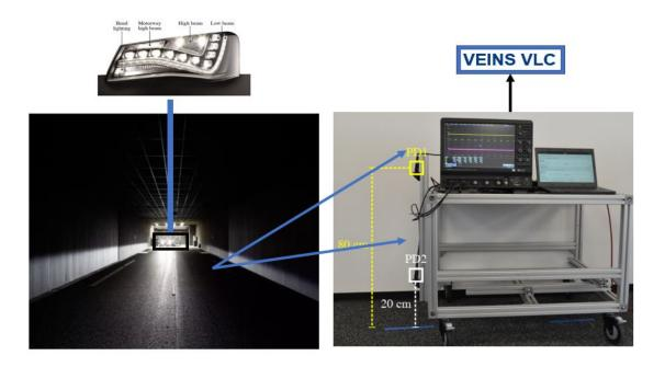
Figure 8.6: Summary of the integration of the empirical model in VEINS-VLC (the images were taken from [110]): the measurements were done at the HELLAâs Lichtkanal company in a light channel room of dimension  $145m \times 11m$ . For the emissions, a real pair of headlights module was used, whereas the receiver side uses two PDs of type PDA100A placed at the same level as the license plate and the tail lights.
