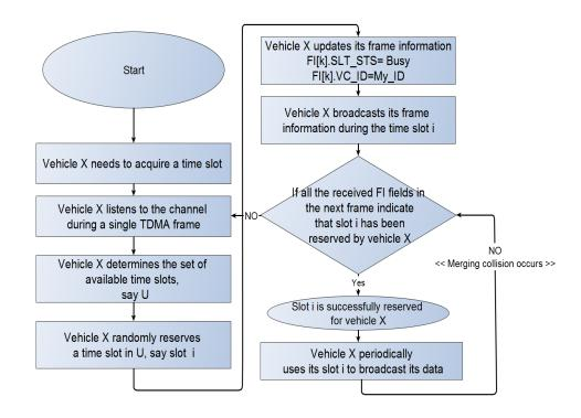
Figure 4.2: DTMAC protocol principle (FI Frame Information)
