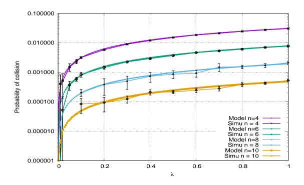
Figure 4.13: Collision probability versus channel load.
