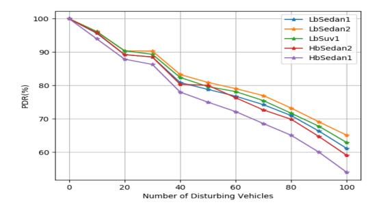
Figure 8.8: V-VLC PDR versus number of disturbing vehicles: Simulation time = 116s; platoon size = 8; platoon inter-vehicle distance = 10 m; Disturbing vehicles' speed = 100 km/h; Platoon vehicles' speed = 15 km/h.
