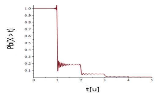
Figure 6.2: Distribution function of the busy period Pb(X > t) for  $\lambda = 0.2$ , t is in time unit (u).
