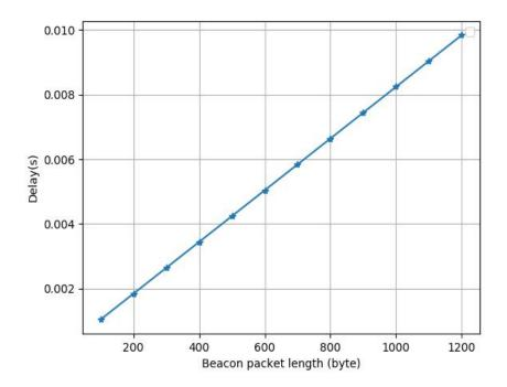
Figure 8.11: V-VLC delay versus platoon beacon packet length
