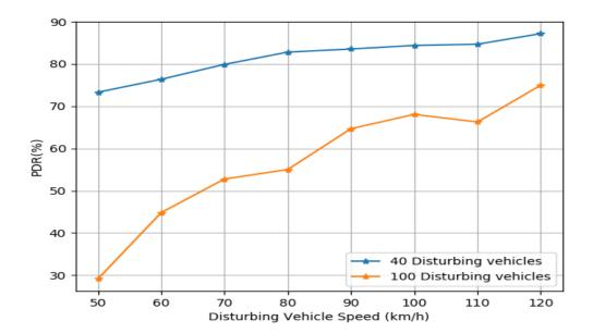
Figure 8.9: V-VLC PDR versus disturbing vehicle speed: Simulation time = 208s; platoon size = 8; platoon inter-vehicle distance = 10 m; Disturbing vehicles' speed = 100 km/h; Platoon vehicles' speed = 15 km/h; Headlight module = "HbSedan2".
