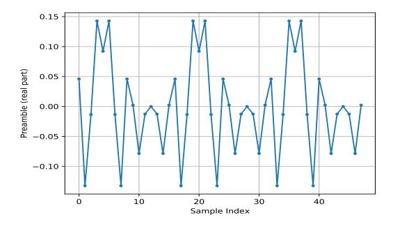
Figure 5.7: Three short preambles (real part).
