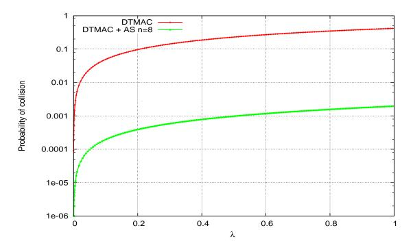
Figure 4.14: Collision probability versus channel load.
