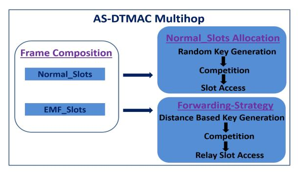
Figure 7.1: AS-DTMAC Multihop Architecture.
