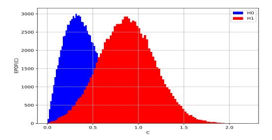
Figure 5.8: Hypothesis testing for OFDM symbol detection: Empirical Probability Distribution Function (EPDF) histogram under  $H_0$  and  $H_1$ . C is the correlation variable at the matched filter output.
