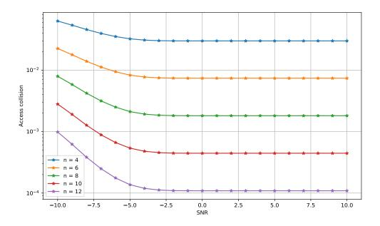
Figure 5.16: Impact of SNR on the access collision
