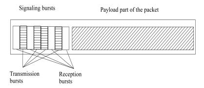
Figure 4.3: Slot structure of the Active Signaling mechanism
