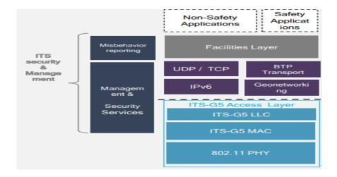
Figure 2.8: ITS-G5 stack architecture [130]
