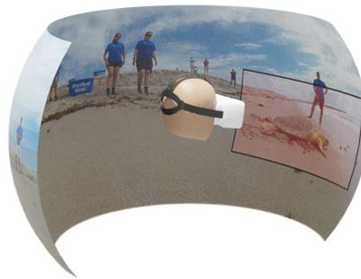
FIGURE 2.4: Layout of a Virtual Reality system with a wearable Head Mounted Display.
