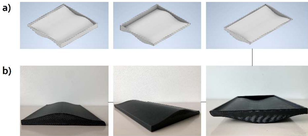
Figure 10.2: a) Schematics of the sinusoidal shaped topography, which is 3D printed in three separated parts and then assembled before being mounted over the support arm and towed in the tank. b) Photos of the middle piece of the 3D printed topography.
