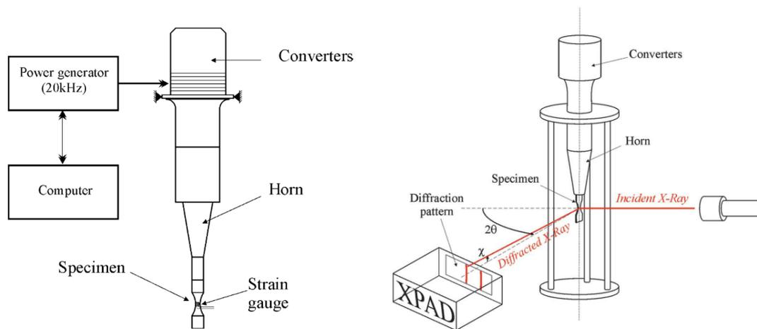
Figure 1.3: Schematic diagram of an ultrasonic fatigue machine.
