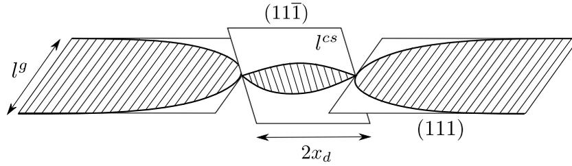
Figure 3.4: An equilibrium configuration during cross-slip via FE mechanism. The process is completed when the constriction separation tends to infinity. In this limit, the dislocation is completely contained in the conjugate plane with separation between the partials  $l^{cs}$  for all  $x$  (figure adapted from Kang et al. (2014)).
