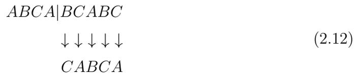
where the vertical line indicates the dislocation position. A so-called intrinsic stacking-fault is formed between the partials due to the missing  $B$  layer:
