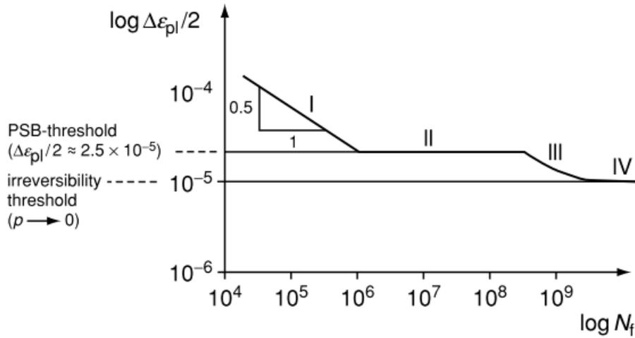
Figure 1.7: Multi-stage life diagram for Type I materials. The numerical values correspond to pure copper.
