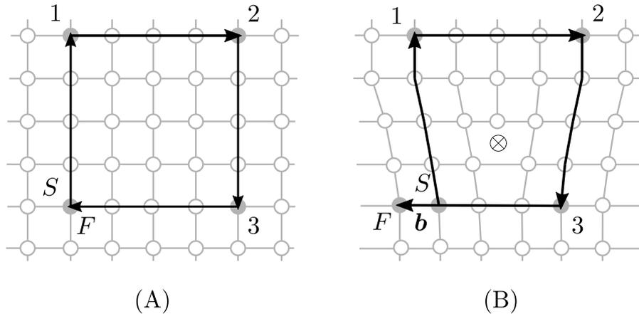
Figure 2.4: Burgers circuits based on the RH-SF convention in: (A) a perfect crystal and (B) a deformed crystal. The  $\otimes$  symbol indicates that the line direction of the edge dislocation points into the page. The starting point of the circuit is denoted as  $S$  and the final point as  $F$ .
