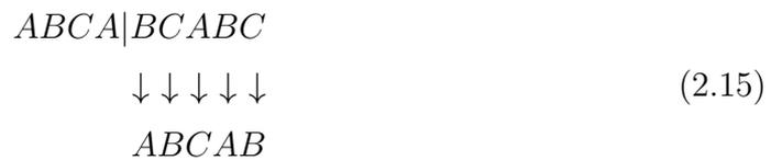
that will spontaneously split into an extrinsic stacking fault made of a double fault of the type  $ABCA|C|B$  involving a faulted prismatic loop. Since the slip provoked by the trailing partial restores the original stacking order of the atomic layers, one says that the leading partial creates a stacking-fault whereas the subsequent movement of the trailing partial removes it.
