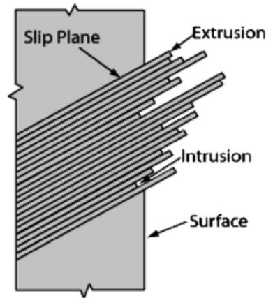
Figure 1.5: Intrusions and extrusions conforming the PSBs.
