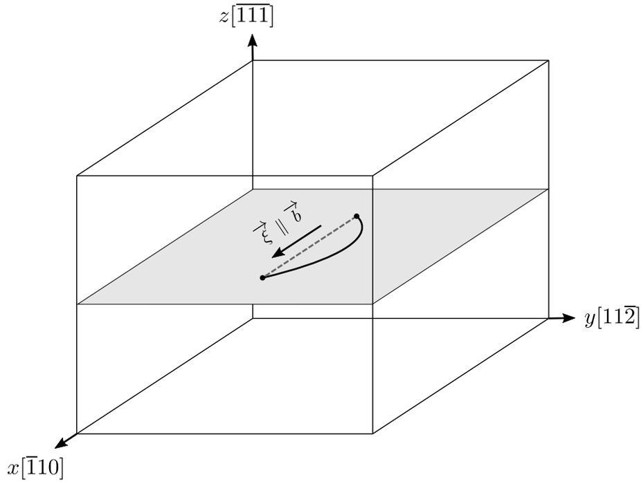
Figure 5.3: Perfect right-handed screw dislocation of length equal to 10,000 Å contained on the  $(\bar{1}11)$  plane. Its Burgers vector and line orientation are parallel to the  $[\bar{1}10]$  direction.
