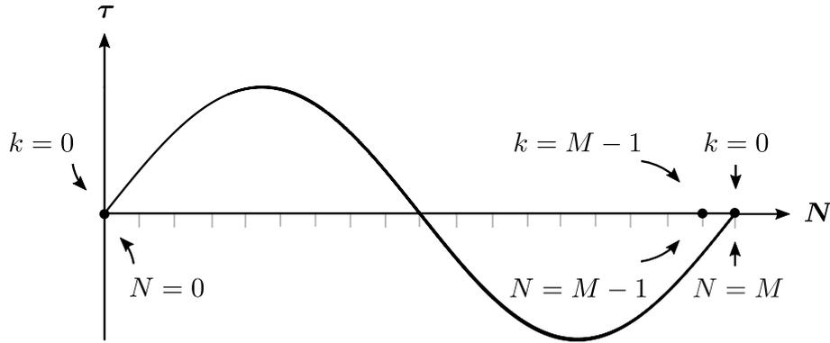
Figure 6.1: Stress cycle applied  $\tau$  as function of the simulation step  $N$ . The loading stage corresponds to a specific part of the cycle characterized by  $k = N \% M$ .
