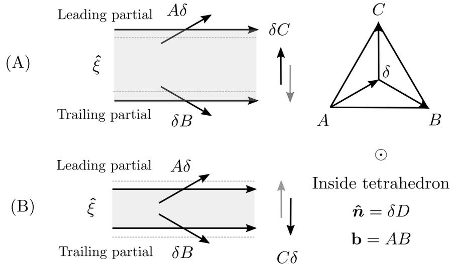
Figure 2.16: View from inside the Thompson tetrahedron of an extended RHS dislocation with Burgers vector  $AB$  under a shearing stress along: (A)  $\delta C$  vs (B)  $C\delta$  affecting only the equilibrium separation. The gray segmented line represents the unstressed dissociation width and the  $\odot$  symbol indicates that the plane normal  $\hat{n}$  points out of the page.
