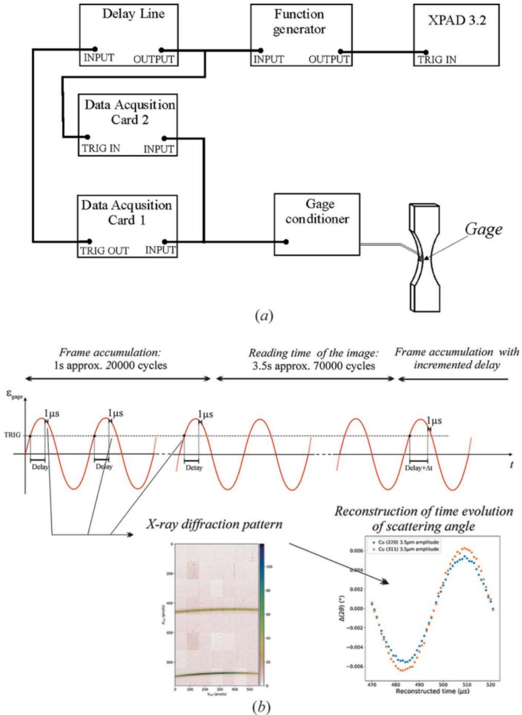
Figure 1.4: Schematic diagram of an ultrasonic fatigue machine.
