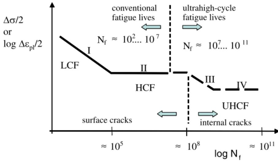
Figure 1.8: Multi-stage life diagram for Type II materials.
