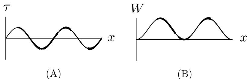
Figure 2.1: Model of [Frenkel \(1926\)](#) for: (A) the shear stress  $\tau$  as function of the relative displacement  $x$  and (B) the periodic lattice potential  $W$  as function of  $x$ .
