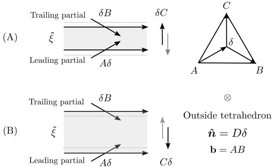
Figure 2.17: View from outside the Thompson tetrahedron of an extended RHS dislocation with Burgers vector  $AB$  under a shearing stress along: (A)  $\delta C$  vs (B)  $C\delta$  affecting only the equilibrium separation. The gray segmented line represents the unstressed dissociation width and the  $\otimes$  symbol indicates that the plane normal  $\hat{\mathbf{n}}$  points into the page.
