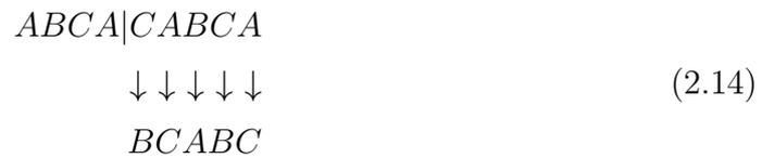
Consider that the leading partial had Burgers vector  $b_2$  instead. In that case, the original stacking order would be transformed to a higher-energy configuration:
