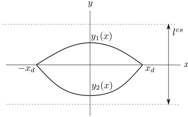
Figure 3.2: The shape of the partials in the cross-slip plane are described by the  $y_1(x)$  and  $y_2(x)$ , and satisfy the boundary conditions  $y_1(\pm x_d) = y_2(\pm x_d) = 0$  (figure adapted from Kang et al. (2014)).
