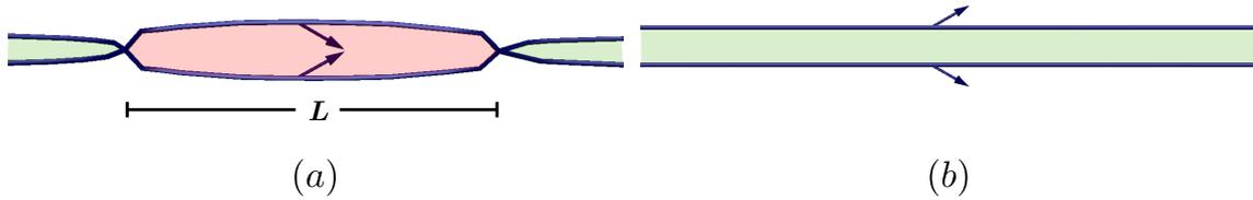
Figure 3.6: Graphic visualization of: (a) an intermediate cross-slip configuration of distance  $L$  between its constriction points and (b) the reference configuration consisting of a relaxed dislocation completely contained on the glide plane. The area shaded in red represents the deviated plane, whereas the region shaded in green indicates the glide plane.
