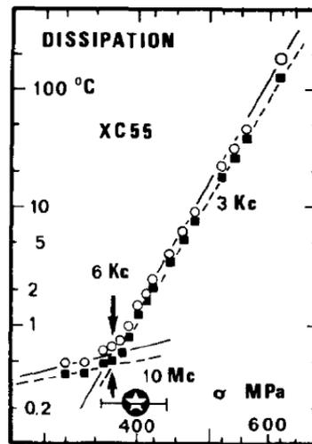
Figure 1.2: Self-heating curve of XC55 steel. *Source:* Luong (1995).
