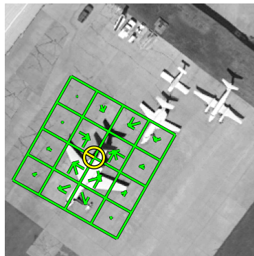
Figure 2.4: The descriptor of a SIFT frame centered at a fixed pixel
