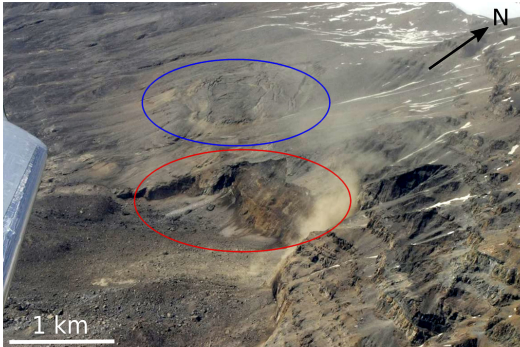
Figure 2 Aerial photograph of the 2017 slide (red ellipse) and the western potential landslide (blue ellipse)
