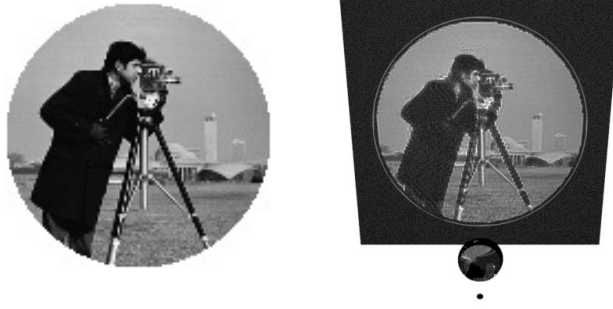
Figure 6.2: Left: target image. Right: simulation of the scene using the appleseed ® rendering engine; the small black disk at the bottom represents the light source.
