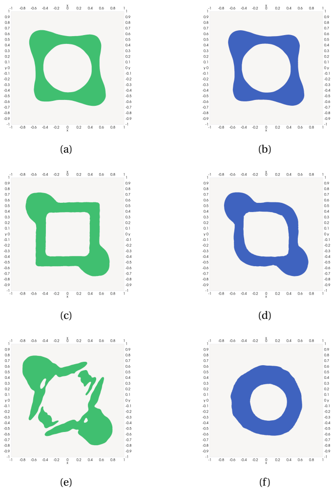
FIGURE 3.4 – Optimal static solution : (a) \theta > 0 : Convexification method; (b) \theta > 0 : Level-set method; (c) \theta = 0 : Convexification method; (d) \theta = 0 : Level-set method; (e) \theta < 0 : Convexification method; (f) \theta < 0 : Level-set method.
