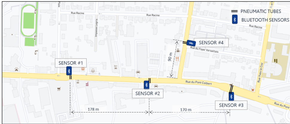
FIGURE 3.1: Sensors placement plan
