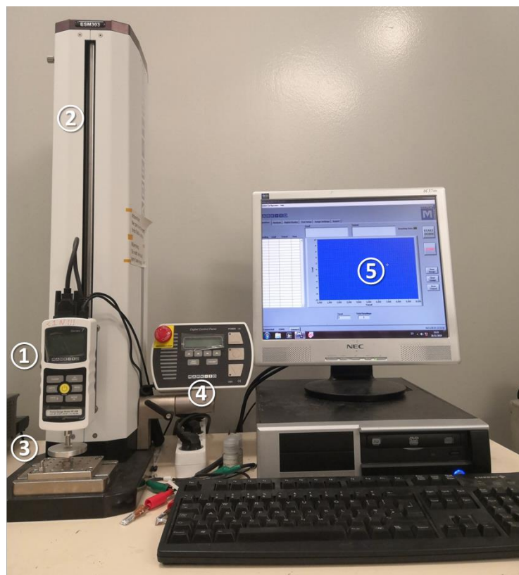
Figure 4-9. The test system consists of a digital force gauge ① (Mark-10, M7-025E, ~1.0 N), a motorized test stand ② (Mark-10, ESM-303E), sample test platform ③ (sample holder and compression plate with diameter of 1.15 cm), control panel ④, and software ⑤ (MESUR gauge Plus).
