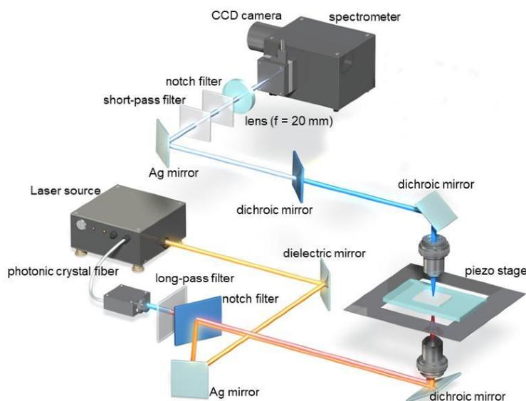
Fig. 1. Experimental setup of ultra-multiplex spectroscopic CARS system.
