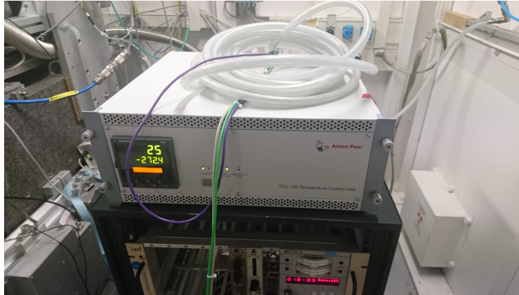
Figure C.2: Anton Paar furnace used for heating up to 200°C in the in situ GISAXS measurements.
