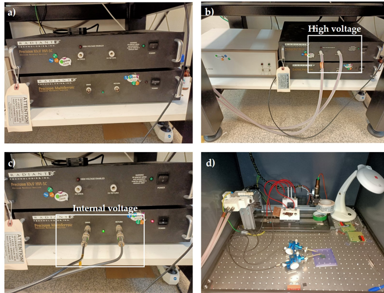
Figure B.2: Images of the ferroelectric measurements setup:(a) Precision 10 kV HVI-SC from Radiant Technologies , (b) External high voltage probe connectors, (c) Internal low voltage probe connectors and (d) characterization test bench with two probes set on the sample.
