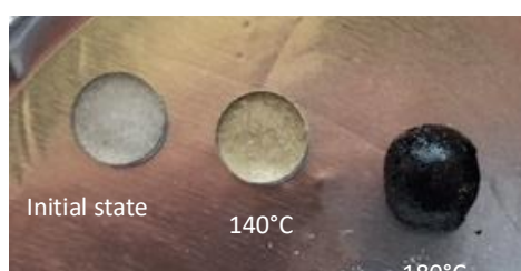
Figure II-38. Ascorbic acid physical evolution after a 5 minutes exposure to different temperatures.
