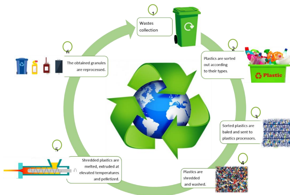
Figure I-3. Plastics recycling process.
