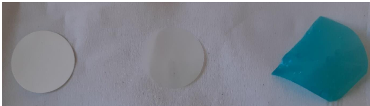
Figure 6. Picture of a porous membrane film before impregnation (left), after impregnation (middle), and of a piece of the SILM after extraction of cobalt from hydrochloric acid media (right).
