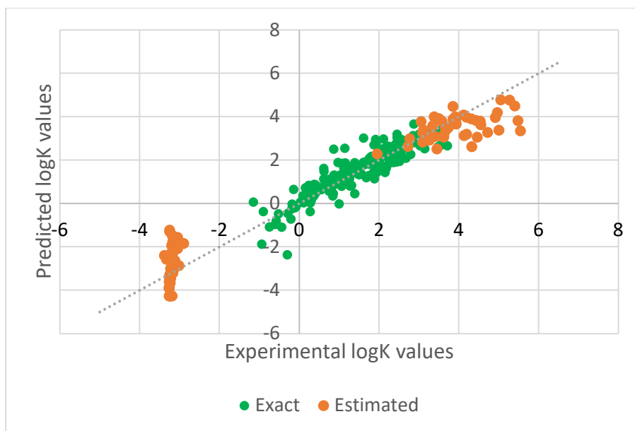
Figure 6.12: Experimental vs. predicted logK values plot of consensus model obtained from 16 SVR models (see Table 1-4). The model's performance is R^2=0.93 and the RMSE=0.62 log units. A gray dotted line corresponds to ideal predictions.
