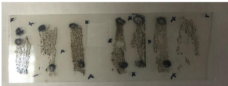
Figure 56: ITO slide containing sludge samples before the MSI analysis.
