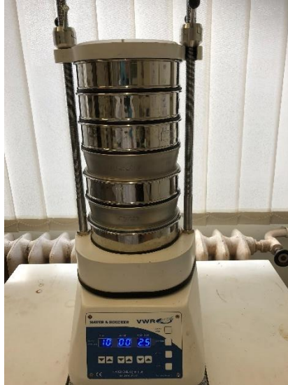
Figure 30: Sludge samples passed through different sized mesh under mechanical stirring.
