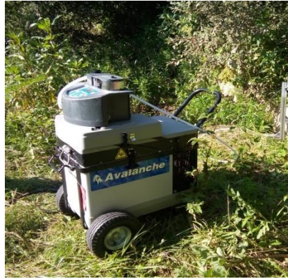
Figure 23: Automatic samplers (Avalanche Teledyne ISCO) used to collect wastewater.
