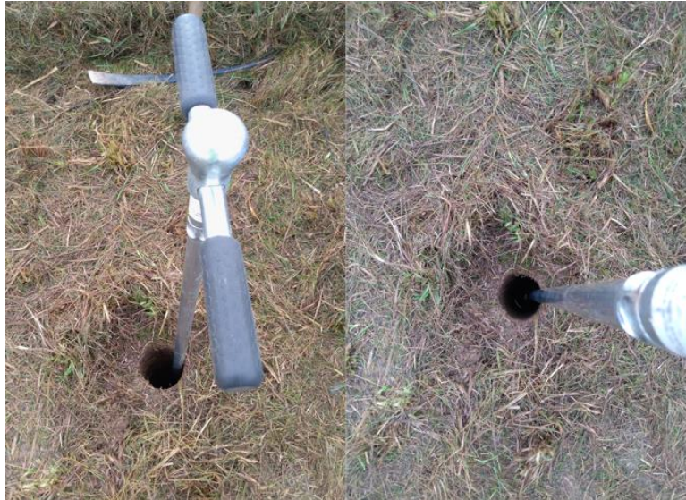
Figure 27: Coring performed using a manual auger.
