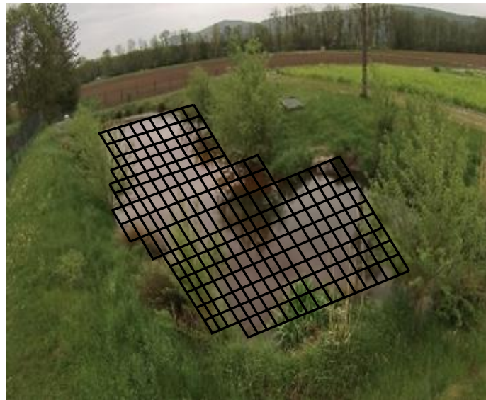
Figure 75: Virtual grid applied on the study site to collect the water depth.
