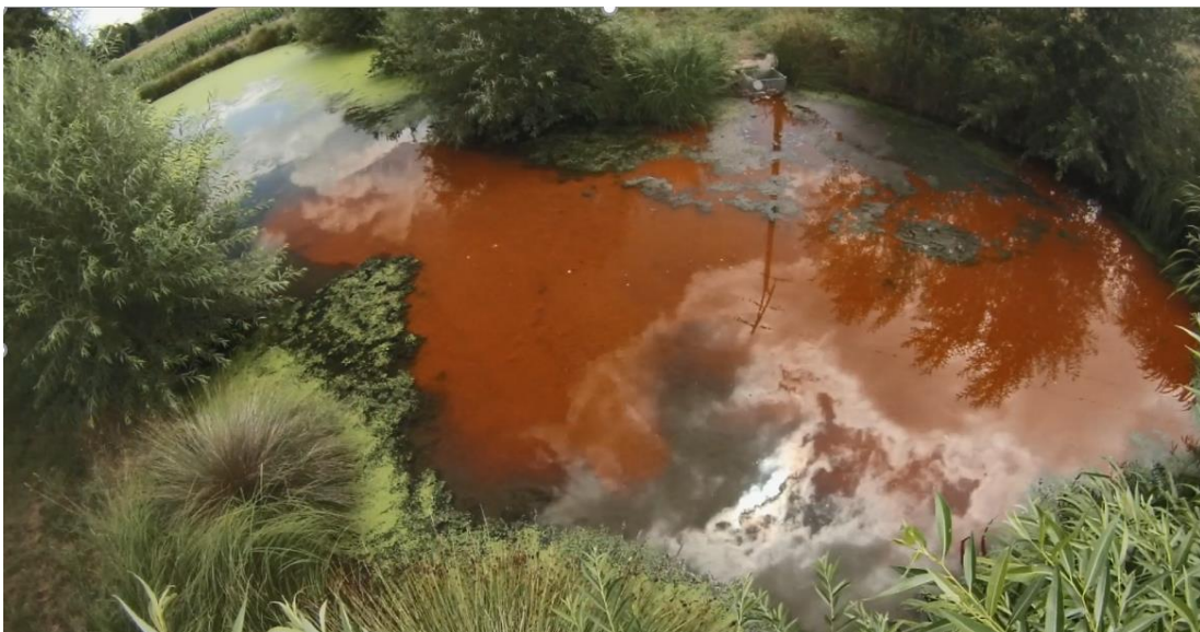
Figure 80: Tracer experiment using sulforhodamine in the artificial pond.
