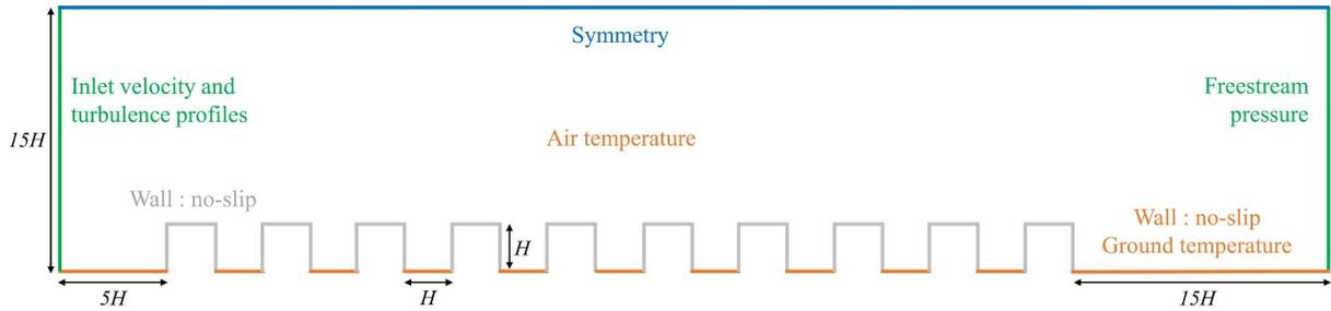
Figure 2.20 – Boundary conditions and domain size
