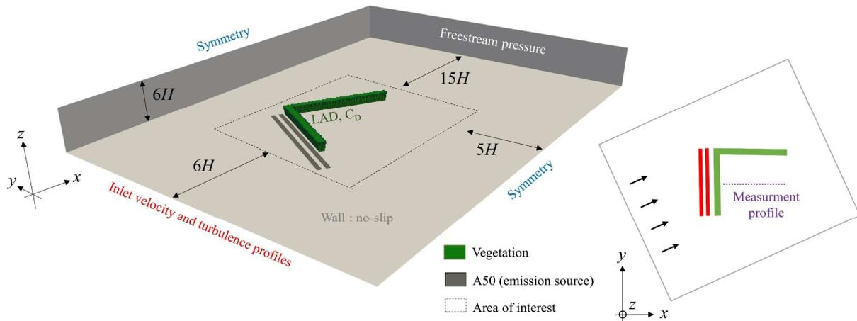
Figure 2.32 – Boundary conditions and domain size.
