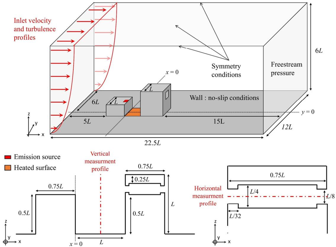
Figure 2.23 – Boundary conditions and domain size.
