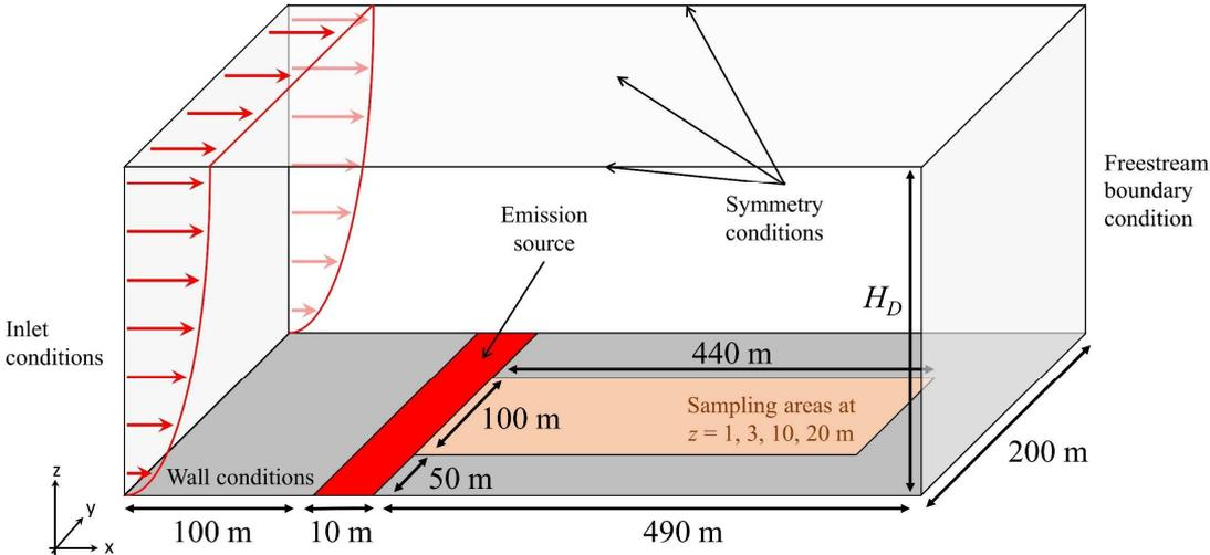
Figure 3.2 – Boundary conditions and domain size.
