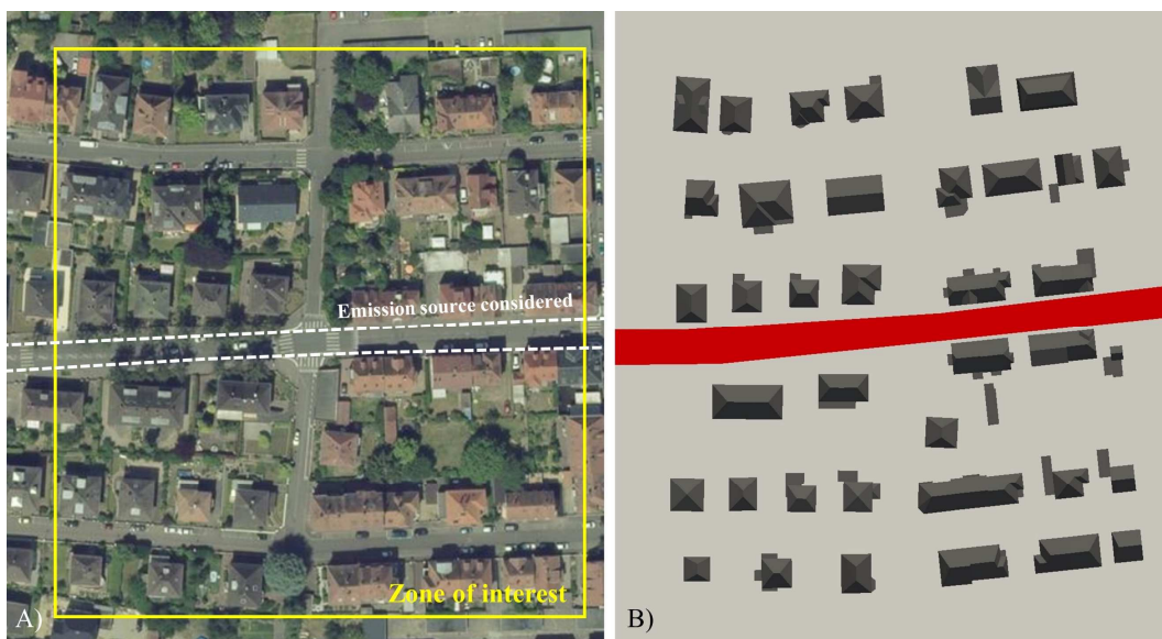
Figure 4.5 – Illustration of (A) the area of Strasbourg modeled with the road considered for the traffic-related emissions (white dashed lines), and (B) the corresponding area built in 3D for the numerical simulations with the emission source (red).
