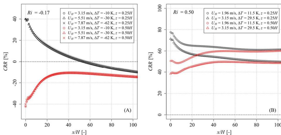
Figure 7.11 – Evolution of the concentration reduction rate for  $Ri = -0.17$  (A) and  $Ri = 0.50$  (B) as a function of wind speed ( $U_H$ ) and thermal variation ( $\Delta T$ ) at  $z = 0.25H$  and  $z = 0.50H$ .
