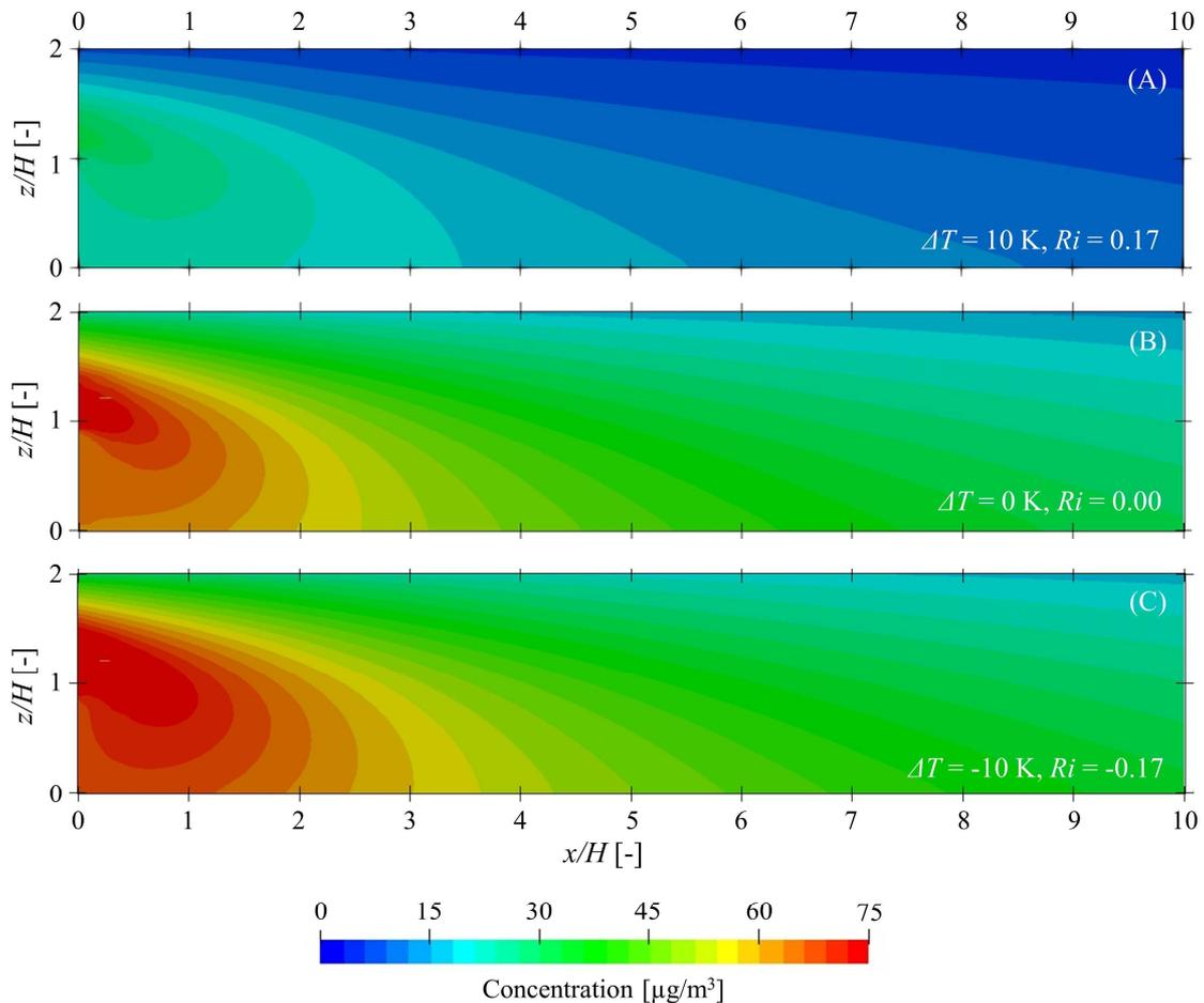
Figure 7.9 – Evolution of the concentration behind the downwind barrier as a function of the temperature variation in the same wind conditions (perpendicular wind,  $U_H = 3.15 \text{ m/s}$ ).
