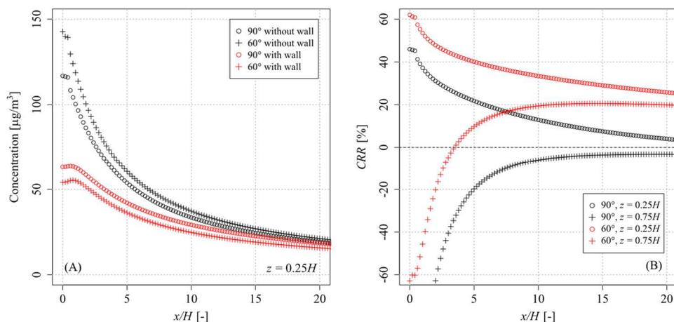
Figure 7.8 – Evolution of the concentrations with and without noise barriers (A) and the concentration reduction rates (B) as a function of the wind direction and for a given wind speed ( $U_H = 3.15$  m/s).
