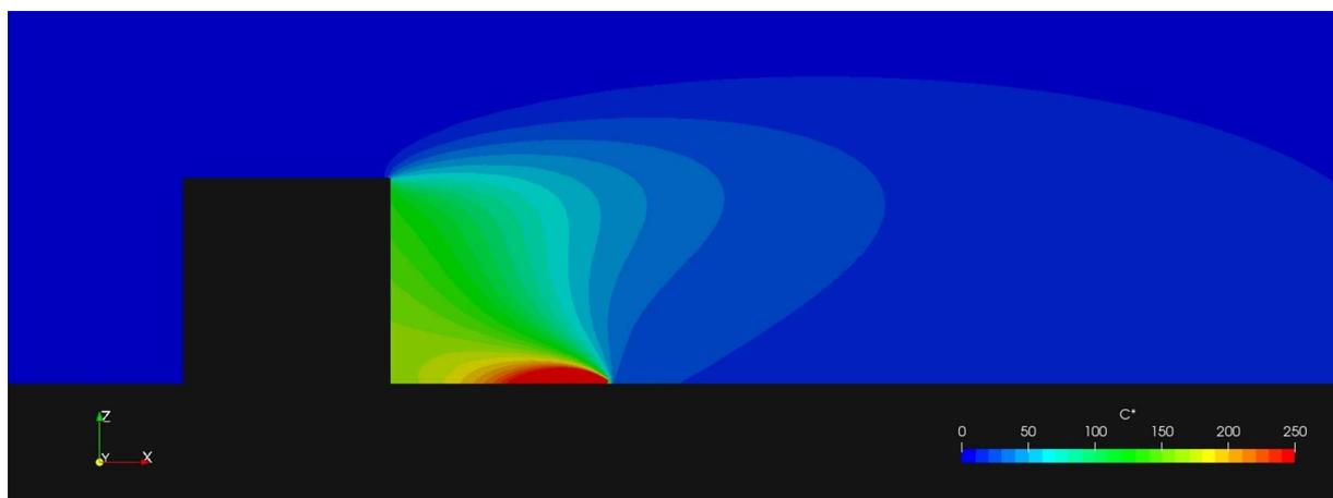
Figure 2.13 – Evolution of dimensionless concentrations after the 2D obstacle with the standard k-ε turbulence model and  $Sc_t = 0.9$
