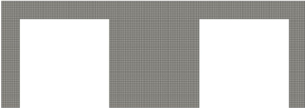
Figure 2.21 – Mesh illustration (1.25 mm for  $z < 2H$  and 5 mm in the rest of the domain).
