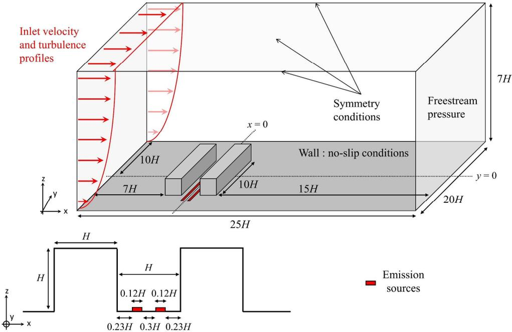
Figure 2.14 – Boundary conditions and domain size.
