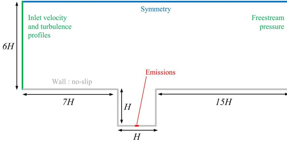
Figure 2.3 – Boundary conditions and domain size.
