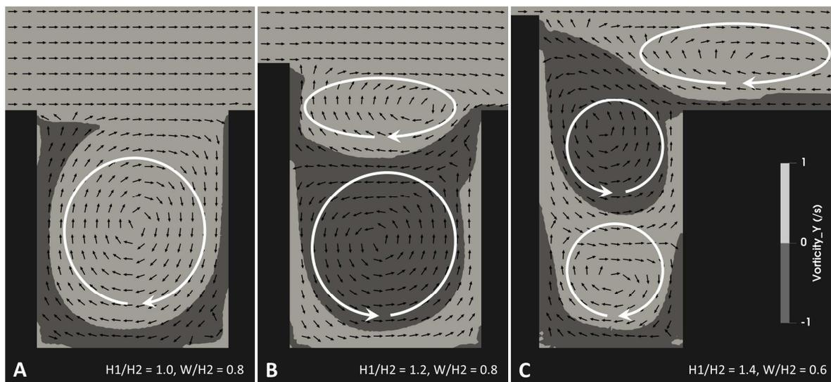
Figure 6.7 – Recirculation patterns, velocity vectors and y-vorticity for different geometric ratios  $H1/H2$  and  $W/H2$ .
