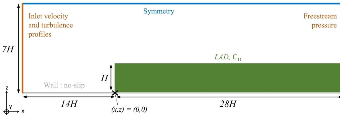
Figure 2.29 – Boundary conditions and domain size.
