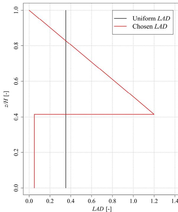
Figure 2.28 – Leaf area density with an uniform density (black line) and a chosen density (red line).
