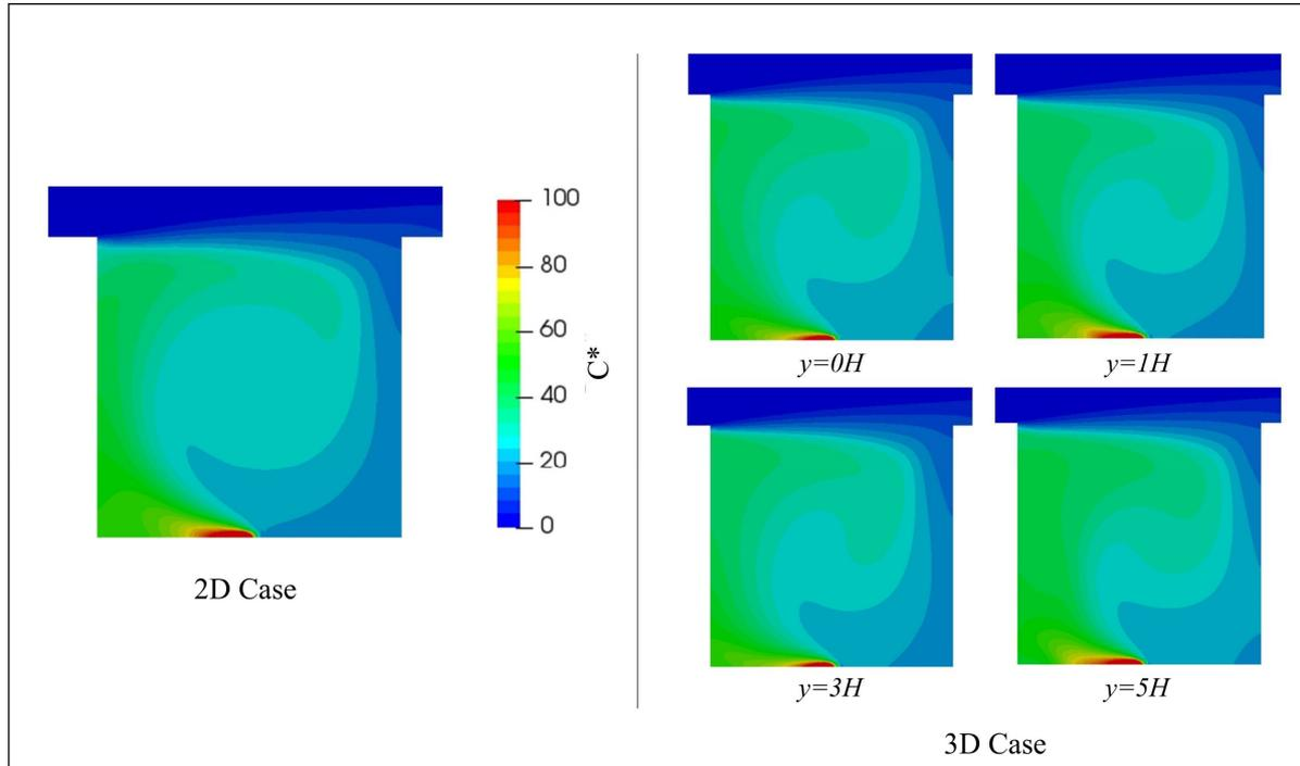
Appendix F.1 – Comparison of the dimensionless concentrations between the 2D and 3D simulation
