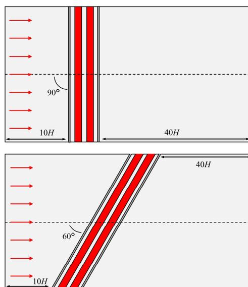
Figure 7.3 – Definition of the wind incidence angle.
