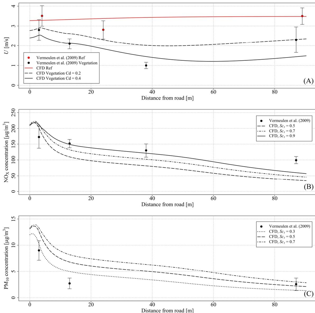
Figure 2.34 – Comparison of the streamwise velocity with and without vegetation and the  $\text{NO}_x$  and  $\text{PM}_{10}$  concentrations between the numerical model and the experimental data of Vermeulen et al. (2009).
