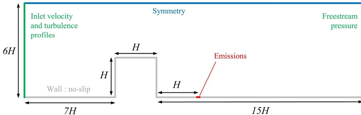
Figure 2.9 – Boundary conditions and domain size.
