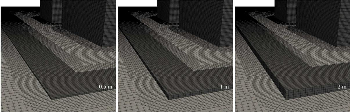
Figure 3.6 – Illustration of the three cases considered with a respective injection height of 0.5 m, 1 m and 2 m.
