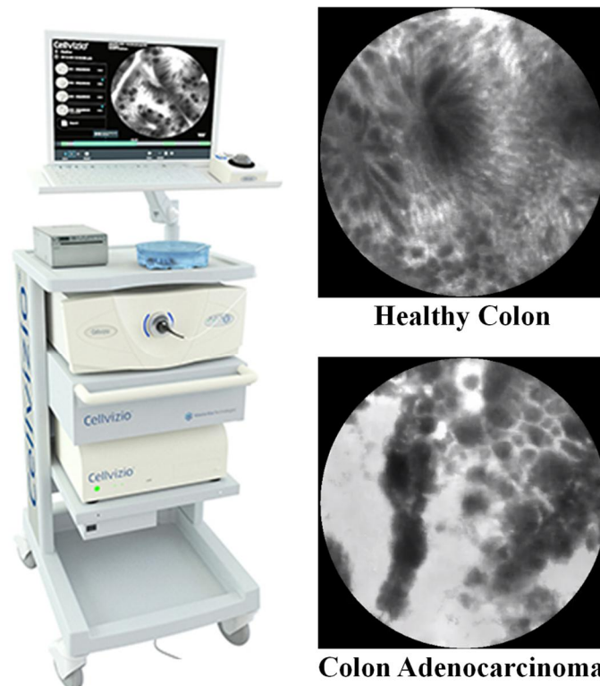
Fig. 1.7. Mauna Kea Technologies Cellvizio flexible microscopic imaging system and confocal laser endomicroscopy image of a healthy colon and of an adenocarcinoma-invaded colon.
