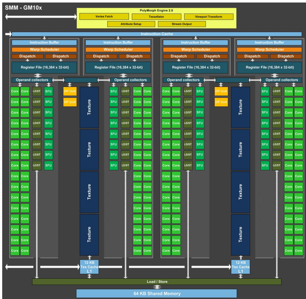
Fig. A2.3. SMM internal structure [5].
