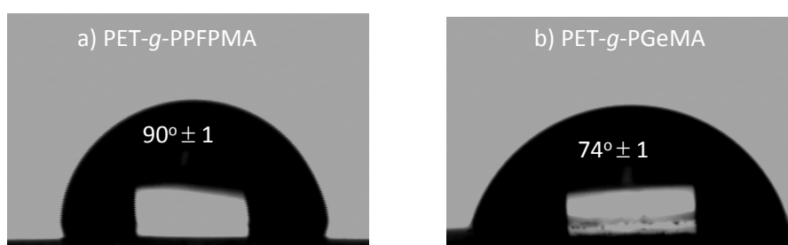
Figure 117. Water contact angle of a) PET- g -PPFPMA, b) PET- g -PGeMA
