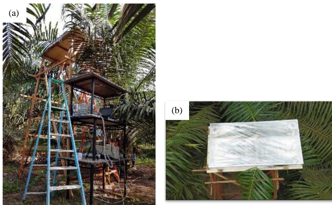
Figure IV.2. Photographs of (a) the whole ^{13}\text{CO}_2 labelling experiment installation in the field and (b) external view of an oil palm leaf enclosed in the labeling chamber.
