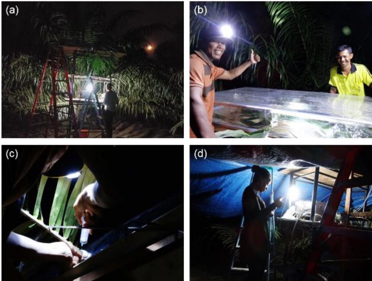
Picture S6. Dark respiration experiment in the field. Pictures of (a,b) the complete installation in the dark, (c) sampling of CO 2 respired inside the chamber using a syringe, and (d) insertion of the CO 2 sampled inside an air tight tube.
