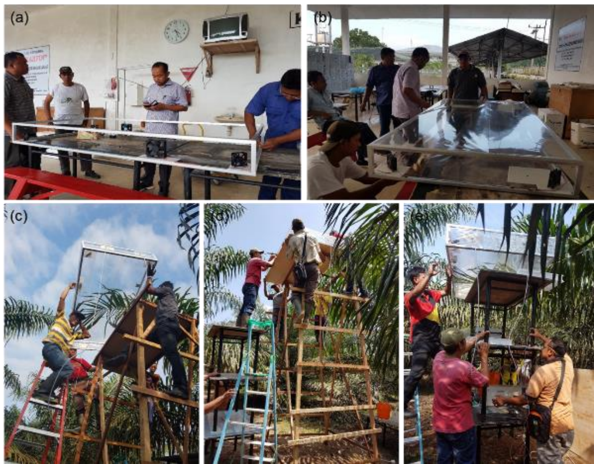
Picture S2. Construction and installation of the labelling assimilation chamber. (a,b) different steps of the construction of the labelling assimilation chamber, (c,d) insertion of the palm inside the chamber, and (e) closing of the chamber.
