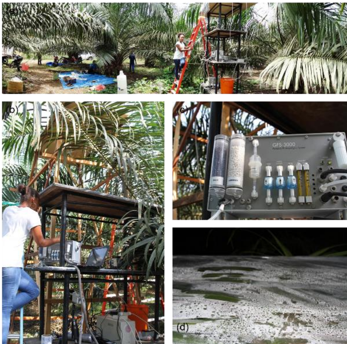
Picture S4. Pictures of the labelling experiment. Pictures of (a,b) the installation and equipment of the labelling experiment, (c) the gas analyzer (WALZ GFS 3000) used for the experiment, and (d) the water condensation on the chamber due to high air temperature and relative humidity inside the chamber.
