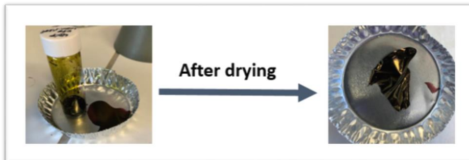
Figure II-45: Sample preparation for DSC.
