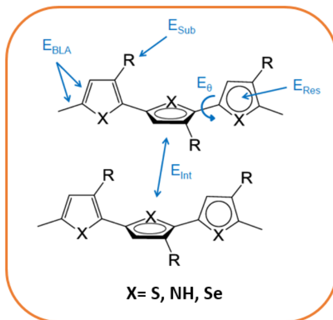
Figure I-12: Structural parameters affecting the bandgap of conjugated materials. 49
