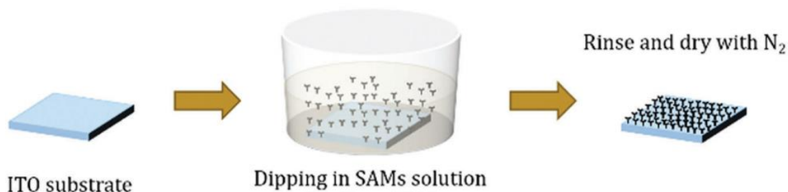
Figure IV-4: Schematic representation for the preparation of the SAMs-coated ITO by immersion. 32
