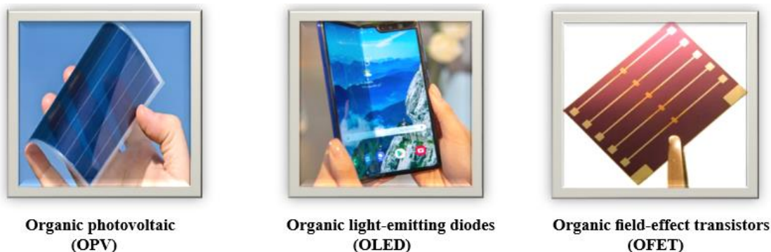
Figure I-4: Examples of some electronic devices based on organic semiconductors.
