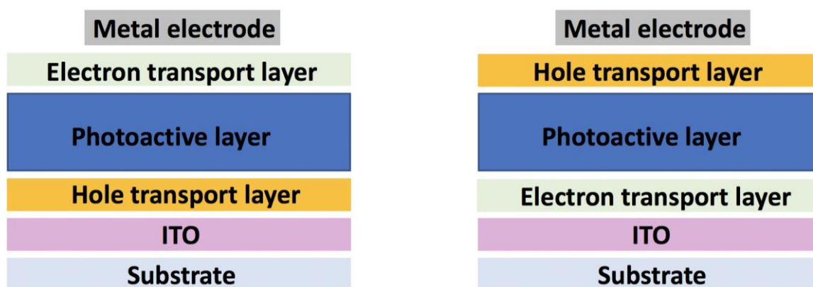
Figure III-3: Typical normal (left) and inverted (right) device structure of OSC.
