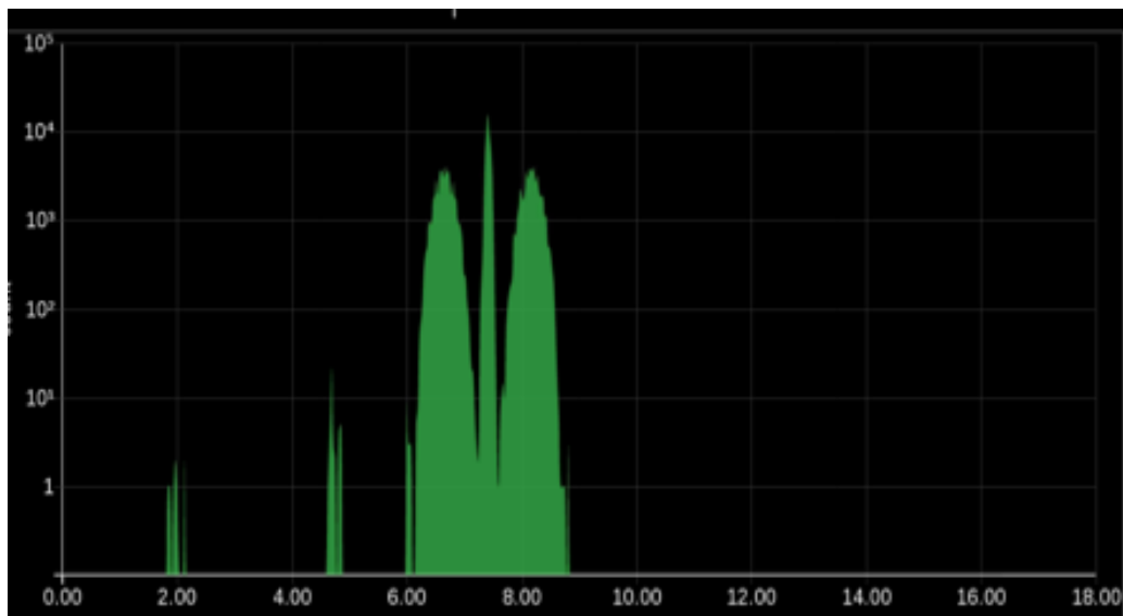
Figure 2.3: Histogram of the packet inter-arrival times at the ingress of the server
