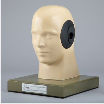
Figure 1.18: ISL dummy head equipped with Type 3.4 ear simulators, called Harry34.
