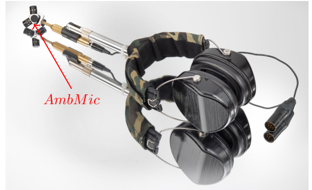
Figure 5.9: Prototype B with the 1 st order ambisonic microphone. AmbMic marks the tetrahedral arranged microphone capsules of the ambisonic microphone.
