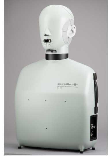
Figure 1.20: B&K head and torso simulator equipped with Type 3.3 ear simulators, called HATS33.
