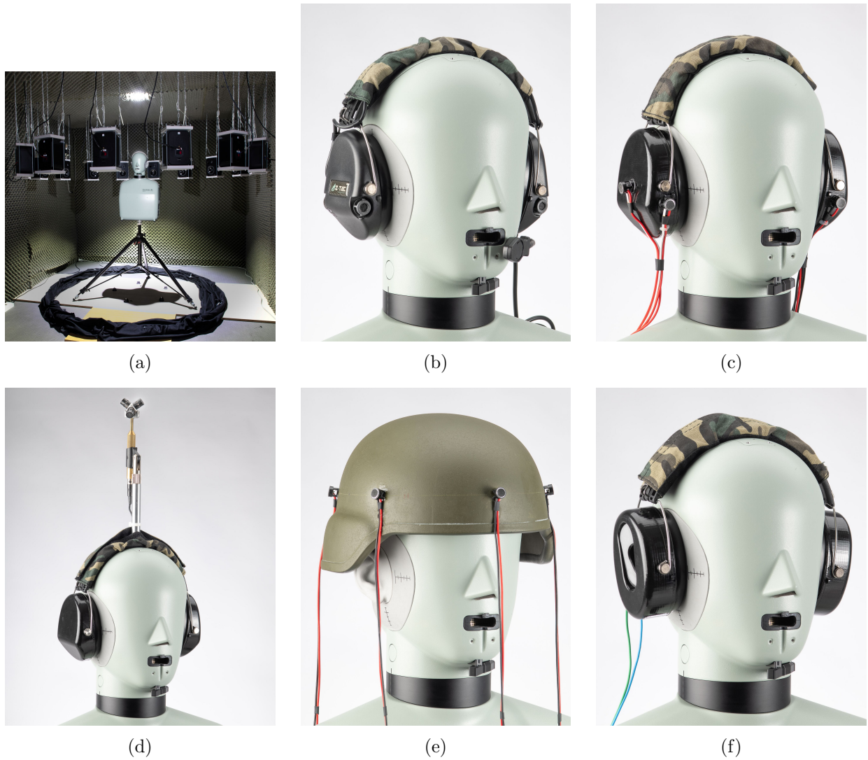
Figure 5.16: Figure 5.16a: Dummy head HATS33 placed in the semi-anechoic chamber, ready for HC0 measurements. According to this setup, the measurement setups for HC1 to HC5 are similar but with the corresponding HPD, resp. prototype put on the dummy head. Figures 5.16b to 5.16f: Close-up views of HATS33 wearing HPD P2 (Figure 5.16b) and Prototype A to D (Figures 5.16c to 5.16f).
