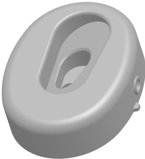
Figure 5.14: 3D model of the left shell of Prototype D. The microphone is integrated in the cutout at the ear canal entrance point of the concha-like cavity. The interactive 3D model is available when reading the electronic version of this document with an suitable PDF reader.
