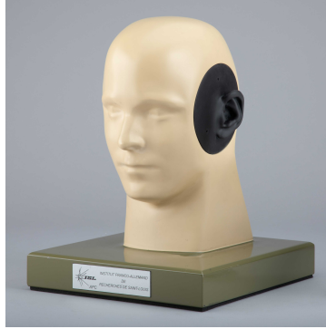
Figure 1.19: ISL dummy head equipped with Type 3.3 ear simulators, called Harry33.
