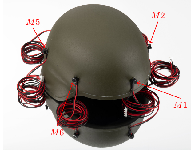
Figure 5.11: Prototype C with labeled microphones. Microphone M3 and M4 are not visible and therefore nor label.
