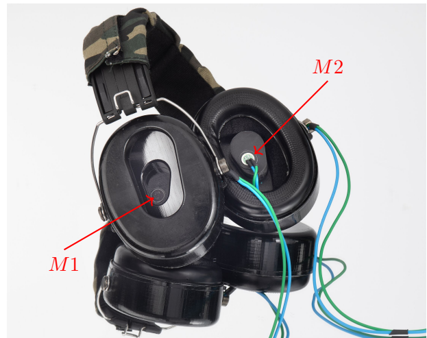
Figure 5.15: Prototype D with labeled microphones in the concha-like geometry of the shell. The interior of the right shell is visible and reveals the back view of microphone M2 .
