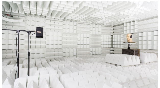
Figure 1.17: View of the anechoic chamber with the loudspeaker on the left side in position \mathcal{A} and the dummy head on the turntable on the right side in position \mathcal{B} .
