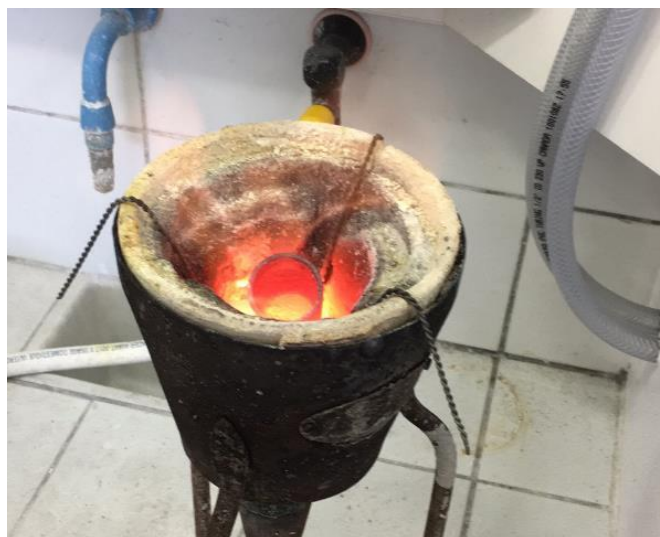
Fig. 3.5 Flame method of preparing glass
