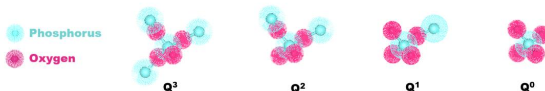
Fig. 3.1 Phosphate tetrahedral sites that can exist in phosphate glasses
