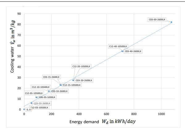
Figure 3.4: Daily cooling water requirements for industrial compressors ( $CF_c = 1$ )
