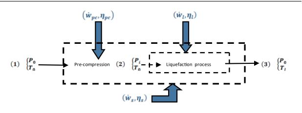
Using the first and the second law over the system, the specific system work  $\dot{w}_s$  can be written, as shown in Equation 3.36.
