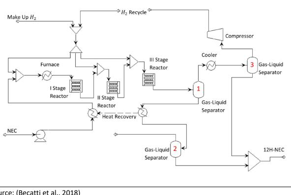
Figure 3.8: Diagram of the hydrogenation process
