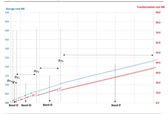
Figure 4.2: Linearization of storage and transformation cost functions
