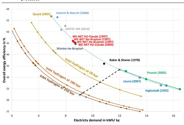
Figure 3.7: Overall exergy efficiency and specific power of current and studied plants and processes
