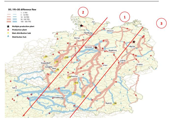
The result flow difference  $D_{ij}$  can be divided into three regions that depend on the multiple production plants with the highest hydrogen production and the change of flow.
