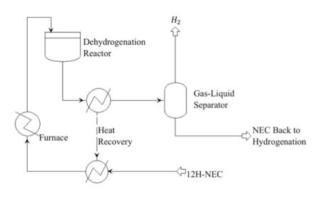
Source: (Becatti et al., 2018) NEC: N-Ethylcarbazole 12H-NEC: Dodecahydro-N-Ethylcarbazole
