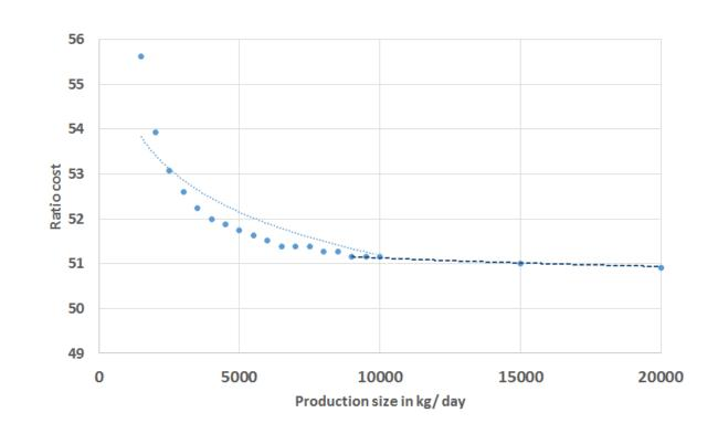
The logarithmic fitting of the results gives a relation between the cost of a given production plant  $Cp_d(p_d)$  of size  $p_d$  and the reference cost  $Cp_1(p_1)$  of the reference plant of size 1000 kg/ day,, as shown in Equation 2.6.
