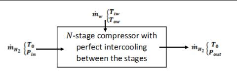
First, the polytropic exponent n is calculated using the specific heat ratio  $\gamma$  and polytropic efficiency  $\eta_p$  (Ozsaban, Midilli, & Dincer, 2011):
