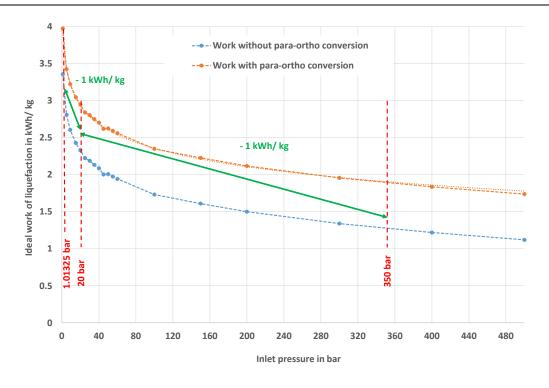
The results show that the ideal work taking into account para and ortho conversion can be modeled as a power function of the inlet pressure with an R-squared of 99.7%, as shown in Equation 3.22:
