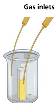
Figure V.13. Bubbling setup of probe solution in Quartz cell.
