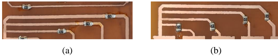
Figure 4.51. SMD resistances mounted on the PCB, (a) parallel to tracks, (b) perpendicular to tracks
