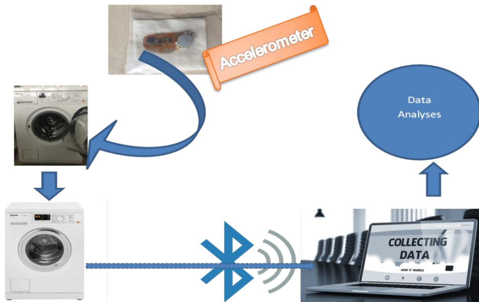
Figure 3.13. Working diagram of the accelerometer used for washing analysis
