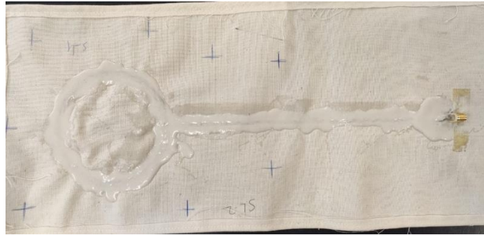
Figure 3.33. Silicon protected textile antenna
