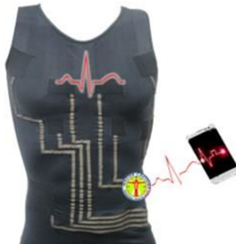
Figure 2.5. HealthWatch ECG t-shirt [99]
