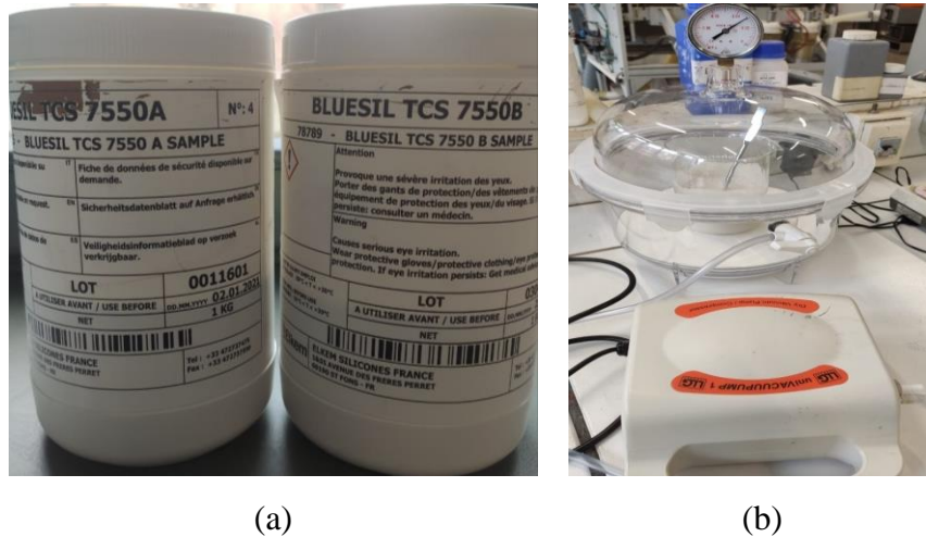
Figure 3.28. (a) Elkem silicon used for the protective layer, (b) vacuum pump with the airtight jar to remove air bubble from solution
