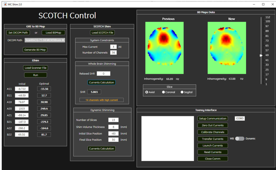
Figure 5.9 – Control interface for SCOTCH to simplify shimming workflow.
