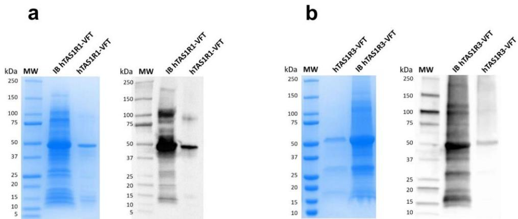
**Figure 2. SDS-PAGE and Western blot analysis of purified inclusion bodies of hTAS1R1- and hTAS1R3-VFTs.** The protein sample, inclusion bodies (IB) and purified hTAS1R-VFTs after gel filtration were separated by 4-15% SDS-PAGE and stained with Coomassie blue or analysed by Western blotting using the anti-His antibody. (a) hTAS1R1-VFT; (b) hTAS1R3-VFT. The molecular weight (MW) standards (BioRad) are shown.
