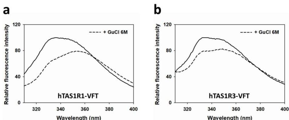
**Figure S5. Chemical denaturation of hTAS1R-VFT proteins followed by intrinsic tryptophan fluorescence.** Addition of 6M guanidinium chloride (GuCl) induced (a) a red shift of 17 nm of the emission maximum and 40% decrease in tryptophan fluorescence intensity for hTAS1R1-VFT and (b) a red shift of 16 nm of the emission maximum and 21 % decrease in fluorescence intensity for hTAS1R3-VFT. These data confirmed that the refolded **hTAS1R-VFT** proteins were properly folded.
