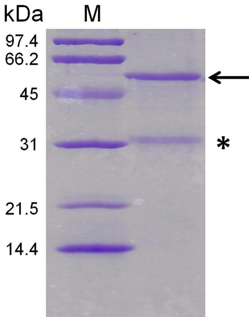
**Fig 2. SDS-PAGE analysis of purified cT1R1-NTD inclusion bodies.** cT1R1-NTD is indicated with an arrow while the star indicates a band corresponding to a N-terminal fragment of cT1R1-NTD. The proteins were separated by 12% SDS-PAGE and stained with Coomassie blue. The molecular mass markers are in lane M.
