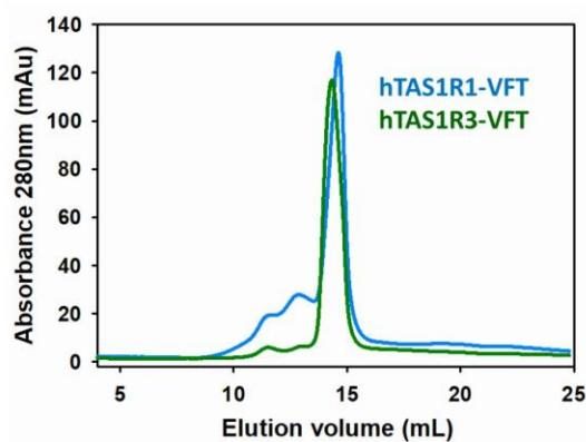
**Figure 1. Gel filtration analysis of refolded hTAS1R1- and hTAS1R3-VFTs.** The chromatography was performed using a Superdex 200 10/300GL column with 50 mM Tris-HCl pH 8.0, 150 mM NaCl, 1 mM DTT and 0.1 mM DDM as elution buffer.
