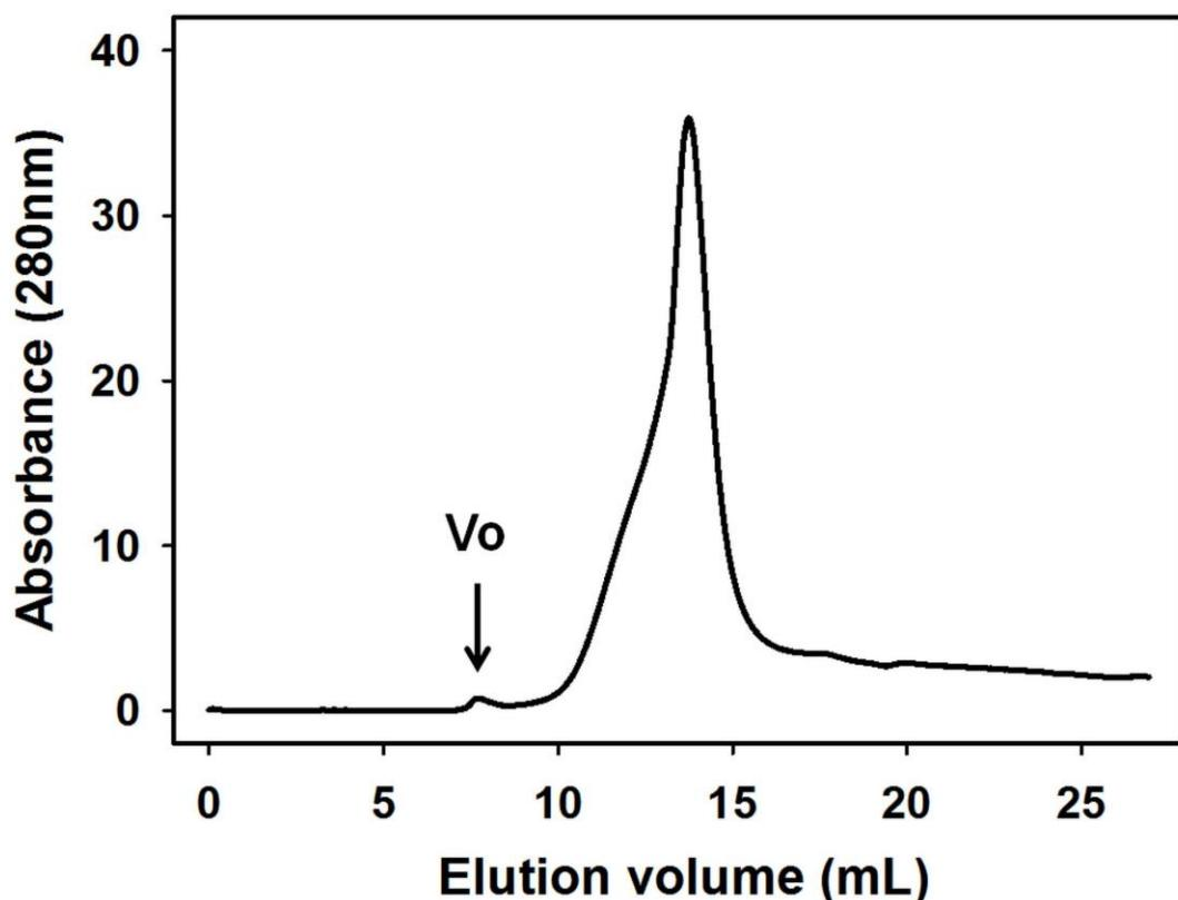
**Fig 3. Preparative gel filtration chromatography of refolded cT1R1-NTD.** Gel filtration was performed using a Superdex 200 column (10 x 300 mm, 24 mL). The column was equilibrated in 50 mM Tris-HCl pH 8.0, 150 mM NaCl, 1 mM DTT, 0.1 mM DDM. The arrow indicates the position of the void volume (Vo).
