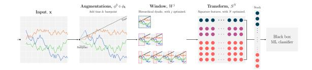
Figure 3.5 – Pictorial representation of the canonical signature pipeline. First, we apply the time and basepoint augmentations to the input paths, then we compute the signature features over dyadic windows, and finally compute the signature features over each dyadic window. These features can now be compiled together and fed into any standard machine learning classifier.
