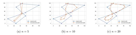
Figure 1.8 – Signature inversion of a sample of the class "8" from the Pendigits dataset
