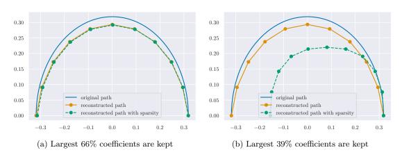
Figure 6.7 – Inversion of the signature truncated at order n = 10 of a half circle, with the complete signature (orange curves) or with a sparse signatures, where the smallest coefficients are set to zero (green curves)
