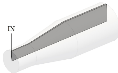
Figure 6.9: Simplified numerical domain with 250mm long upstream extension used in RANS.
