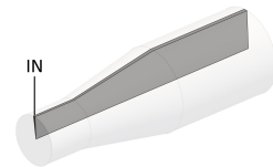
FIG. 11: Simplified numerical domain with 250 mm long upstream extension used in RANS.
