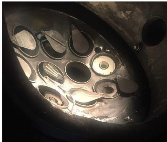
Figure 3.4: Image of the MBE growth chamber of the lab, showing the cells and their effusion cell shutters.
