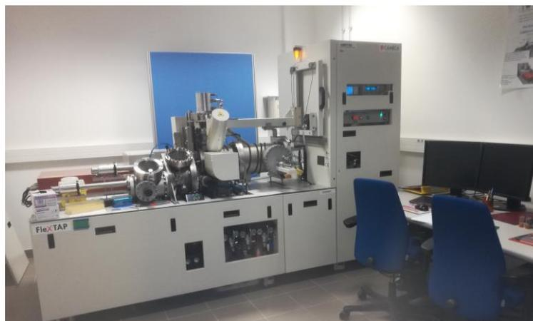
Figure 3.34: CAMECA FlexTAP APT system available in the NanoCharacterisation PlatForm (PFNC).
