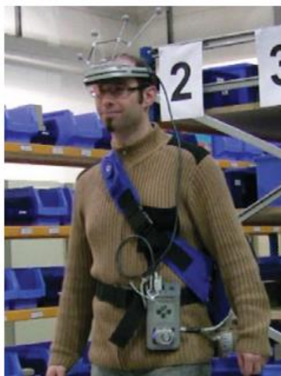
Figure 9 - Dispositif pick-by-vision , utilisant le Microvision Nomad ND2000 (Schwerdtfeger et al., 2009) © [2009] IEEE.
