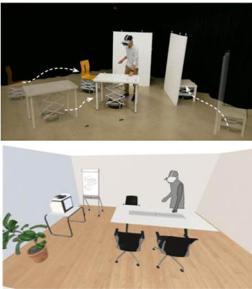
Figure 4.6: RoomShift [Suzuki et al., 2020]: Mobile Robots moving furniture around the VR arena.
