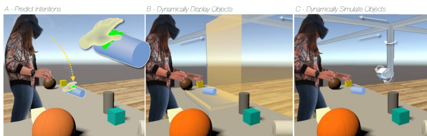
Figure 1.3: My approach is to (A) anticipate the users intentions, to (B) provide them with their object of interest. An interface could even reconfigure itself to (C) simulate the object of interest with similar haptic properties.
