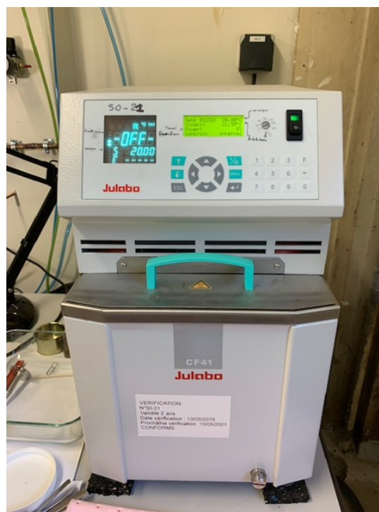
II.21b Cryothermostat JULABO CF 41
