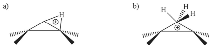
Figure I- 15. a) Edge protonated cyclopropane (EPCP). b) Corner protonated cyclopropane (CPCP, or methyl-bridged structure). [36,60]
