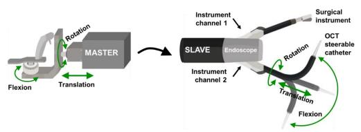
Figure 4.6 Relation of the degrees of freedom in the instrument and the master controller. The system works in Master-Slave configuration.
