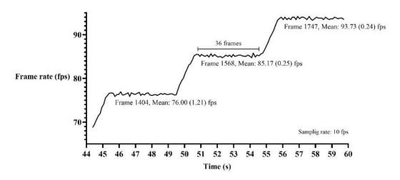
Figure 3.18 Frame rate versus time showing the mean and standard deviation of the frame rate, the number of collected frames, the chosen frame for NURD analysis in which there is mean and the standard deviation of the speed.
