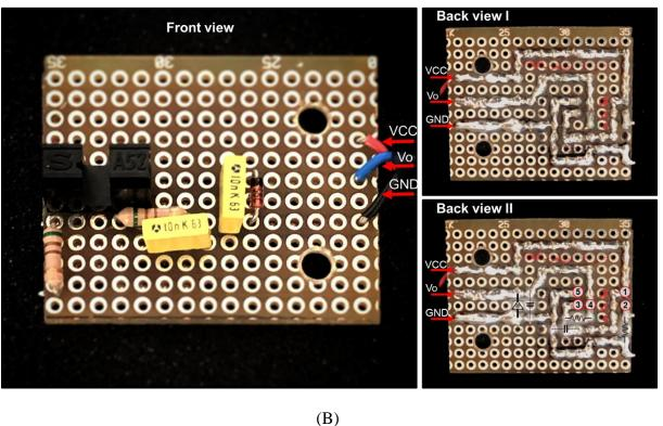
Figure F.4 (A) Matrix board wiring of the synchronization sensor of the helical scanner. (B) Back view schematic drawing. (B) Pictures of the wired circuit, front and back views.
