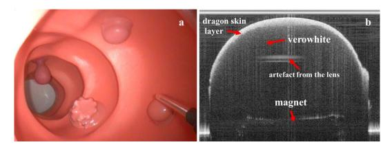
Figure 5.12 (A) White-light endoscopy image of artificial colon with phantoms, (B) benchtop OCT image of polyp phantom.
