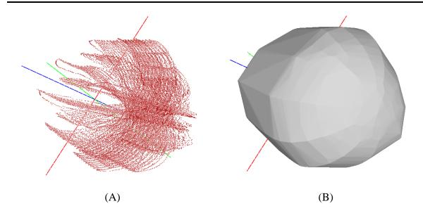
Figure 4.20 Point cloud rendered in MeshLab (A) resulting in an estimated area of  $209.69 cm^2$  and a volume of  $255.29 cm^3$  by using the convex hull filter (B). Axis x, y and z in red, green and blue colors respectively.
