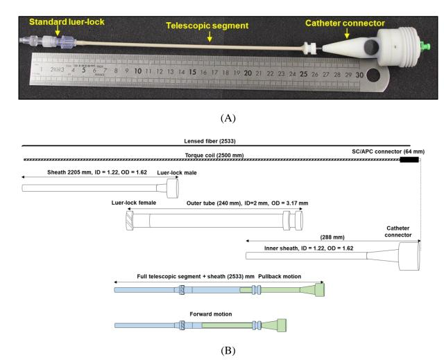
Figure 3.9 Description of the telescopic segment and its internal components.
