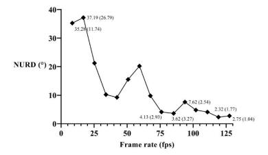
Figure 3.20 NURD versus speed of rotation in frames per second (fps) for regular OCT catheter.
