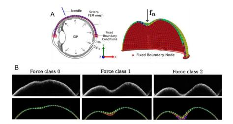
Figure 1.30 (A) Deformed model of the sclera, (B) Force classification based on simulation-trained neural networks from OCT images. Adapted/reprinted by permission from Springer Nature: Int J CARS. Force classification during robotic interventions through simulation-trained neural networks by Mendizabal, A., Sznitman, R. & Cotin, S. © 2019 [269].
