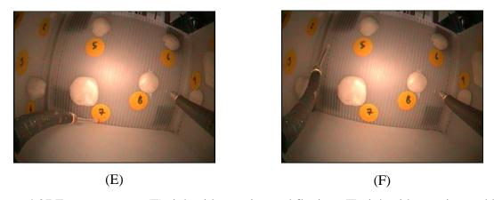
Figure 4.27 Free space test: (E) right side rotation and flexion, (F) right side rotation and left side flexion.
