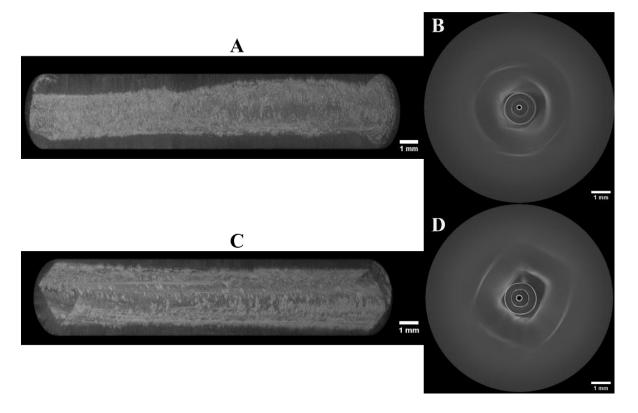
Figure 4.23 3D reconstruction of the rectangular tube by performing regular pullback scanning (a) at 125 fps, and robotic pullback scanning (c) at 125 fps, the sum of the frames corresponding to the regular pullback scanning (b) and the sum of the frames corresponding to the robotic pullback scanning (d).
