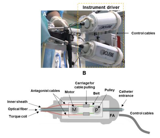
Figure 3.12 Instrument module to provide bending to the distal end of the catheter.
