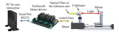
Figure 2.7 Translation stage of the reference arm and its connection with the motor driver and user PC.
