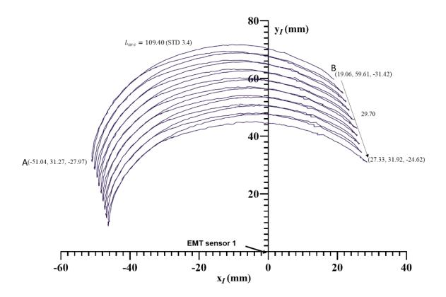
Figure 4.16 Position of the tip of the OCT catheter when performing repetitive trajectories over the range of -90° to 90° of bending angle and a translation of  $\approx$ 30 mm (XY view).
