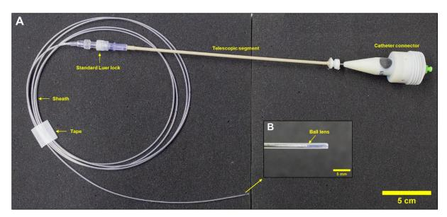
Figure 3.10 Non-steerable OCT catheter with proximal connector, telescopic segment and protecting sheath.
