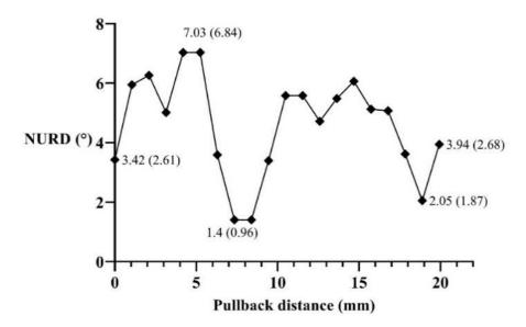
Figure 3.29 Rotational distortion versus pullback scanning distance for regular pullback and with steerable catheter.
