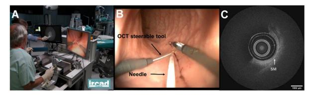
Figure 5.16 In vivo test: (A) The clinician manipulates the steerable OCT catheter by teleoperation. (B) Real time visualization of the colon wall in a living swine; Endoscopic view, (C) OCT view. The submucosa is shown as the brightest layer in the OCT image.
