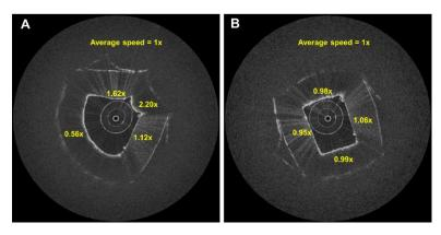
Figure 3.15 Non-uniform rotational distortion in OCT images, (A) image taken at the speed of 1000 rpm and (B) 5000 rpm.
