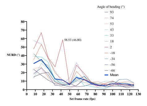
Figure 3.23 NURD versus speed of rotation considering the full range of angle of flexion of the steerable catheter.
