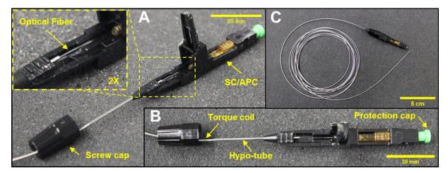
Figure 3.3 Assembly of the SC/APC fast mount proximal connector. (A) Optical fiber and torque coil placed into the SC/APC connector. (B) Hypo-tube covering the torque coil to avoid loops during rotation; green cap to protect the ferule of the connector. (C) Complete assembly of the optical probe.
