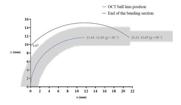
Figure 4.12 Trajectory of the OCT ball lens when the tool enters the channel in retraction maximum bending angle with respect to beginning of the flexible section,  $I = 9.67 \, mm$ ,  $\beta \, [0^{\circ}, 90^{\circ}]$ ,  $\Delta T \geq \Delta T \max$  and  $\emptyset = 0^{\circ}$ .
