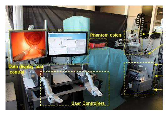
Instrument drivers Sheath and optical probe 3D scanners actuators Endoscope Processor OCT System
