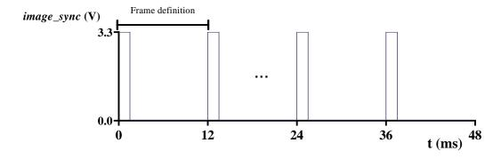
Figure 3.6 Synchronization of the Frame acquisition through the *image\_sync* signal for endoscopic imagine.
