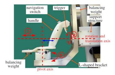
Figure 4.5 Close-up view of one of the master interfaces, © 2018, IEEE [98].
