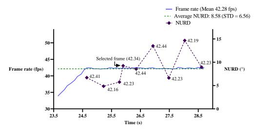
Figure 3.19 NURD versus speed of rotation in frames per second (fps) for regular OCT catheter.
