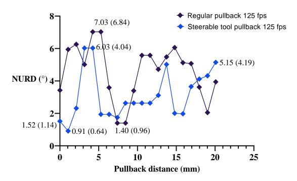
Figure 4.21 Rotational distortion versus pullback scanning distance for tool pullback with steerable catheter (mm).
