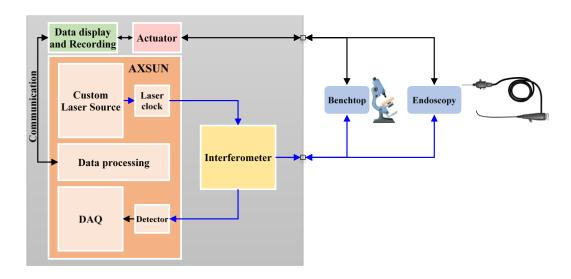
Figure 2.1 General scheme of the OCT Imaging Console (OCT-IC).
