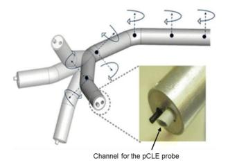
Figure 1.31 The 7-DoF robotic articulated endoscope. It has two operating channels: the camera and interchangeable instruments such as a pCLE. Adapted/reprinted by permission from Springer Nature: Surgical Endoscopy. Robot-assisted transvaginal peritoneoscopy using confocal endomicroscopy: a feasibility study in a porcine model by Newton RC et al. © 2012 [270].
