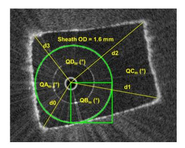
Figure 3.17 Measuring process of the experimental values for the angles  $QA_m$ ,  $QB_m$ ,  $QC_m$  and  $QD_m$ . Tools provided by the ImageJ software were used on the OCT images to perform all the measurements.
