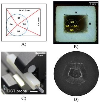
Figure 3.16 Rectangular shape used to measure the rotational distortion. The picture A) represents the geometrical model, B) the 3D printed target and the actual angles, C) the target in place with the OCT catheter, D) OCT image of the target at 25 fps.
