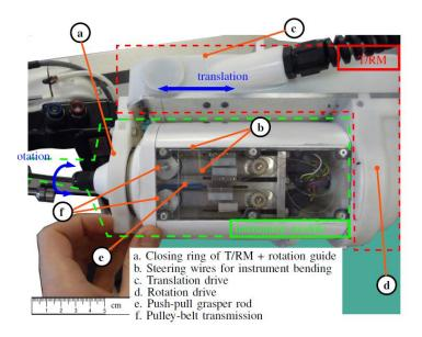
Figure 4.2 Instrument module to perform actuation of the deflection in one plane of the surgical instrument, © 2018, IEEE [98].
