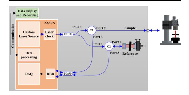
Figure 2.13 Experimental setup for SNR optimization.
