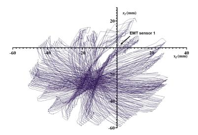
Figure 4.18 Position of the tip of the OCT catheter when performing repetitive trajectories over the range of -90° to 90° with a translation of  $\approx$ 30 mm and a rotation range from 0 to 360° (XZ view).
