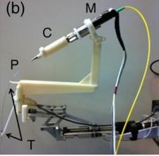
Figure 1.26 Robot-assisted three-dimensional registration for cochlear implant surgery using a common-path swept-source optical coherence tomography probe (CP-SSOCT). (A) Picture of the robotic platform. (B) Close-up of the robotic arm with the mounted rotary motor (M), casing (C), 21G tubes for restricting lateral motion (T), and CP-SSOCT needle probe (P) [239].
