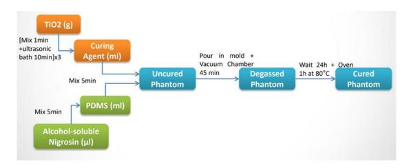
Figure E.3 Fabrication procedure
