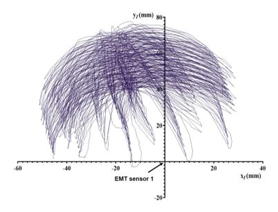
Figure 4.17 Position of the tip of the OCT catheter when performing repetitive trajectories over the range of -90° to 90° with a translation of  $\approx$ 30 mm and a rotation range from 0 to 360° (YX view).
