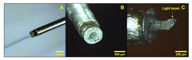
Figure 3.2 Assembly process of the optical probe. (A) The optical fiber core is inserted into the driveshaft. (B) The lensed is fixed just outside of the driveshaft. (C) Lateral view of the ball lensed showing reflected test light.
