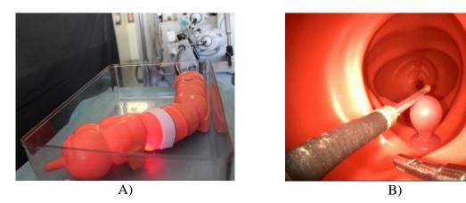
Figure 5.1 Ascending colon model LM107C used for test, (A) external view, (B) endoscope view and peduncular polyp.
