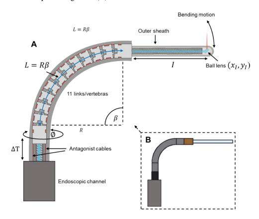
Figure 4.7 Active catheter of piecewise constant curvature, consisting of 11 vertebrae, L is the length of the vertebrae systems.
