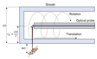
Figure 3.4 Helical scanning implements rotational and translational motions.
