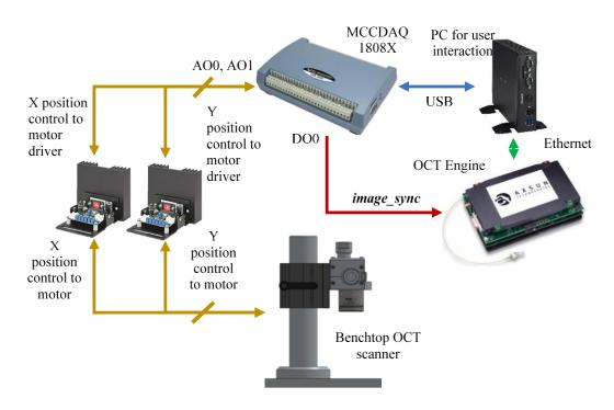
Figure 2.9 Electrical connection for control and communication of the Benchtop imaging system, motor drivers, MCCDAQ, AXSUN OCT engine and the PC for user interaction.
