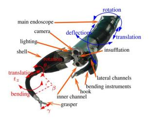
Figure 1.17 Distal part of the endoscopic platform. © 2018, IEEE [98].
