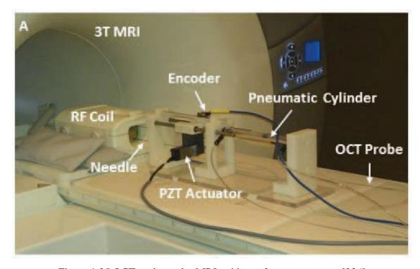
Figure 1.25 OCT probe under MRI guidance for neurosurgery [236].
