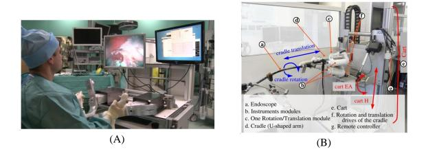
Figure 1.18 (A) Master interface and (B) slave interface (B) of the STRAS robot. © 2018, IEEE [98].
