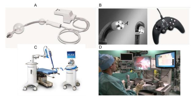
Figure 1.16 (A) Aer-O-Scope, (B) Endotics system, (C) Flex® Robotic System and (D) ISIS/STRAS system.
