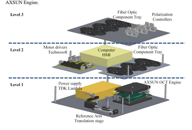
Figure 2.2 Exploded-view of the OCT-IC and its components.
