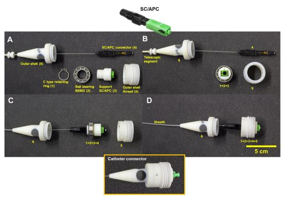
Figure 3.8 Catheter connector assembly.
