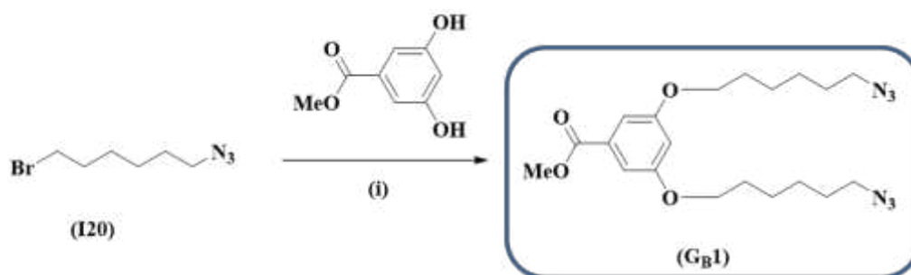
Scheme 4-13. Reaction pathway of G B1 . Reagents and conditions: (i) DMF, \text{K}_2\text{CO}_3 , KI, 80 °C.
