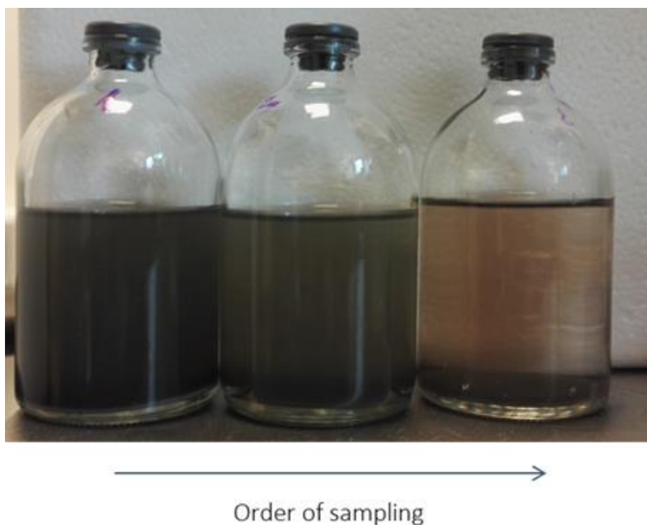
Figure 46: Visual observation of a lack of homogeneity in the BHP
