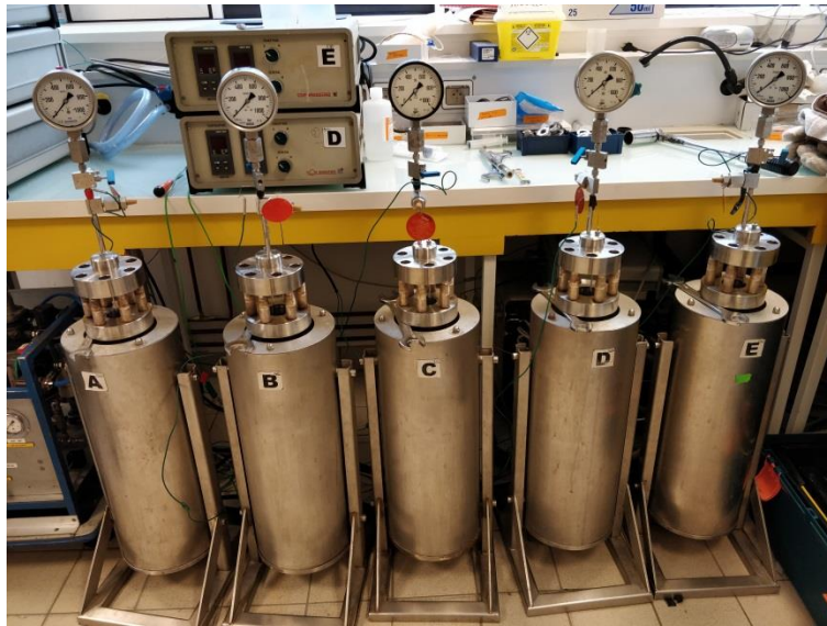
Figure 35: Photo of the five discontinuous HP/HT incubators of the LM2E and their regulators/generators at the beginning of the HPBioHyd project and schematic representation of one device
