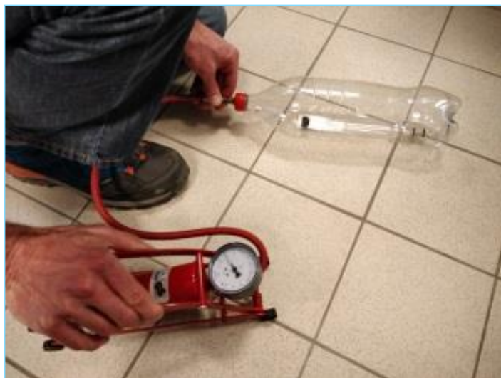
Figure 40: Example of joint behavior observation in dry overpressure
