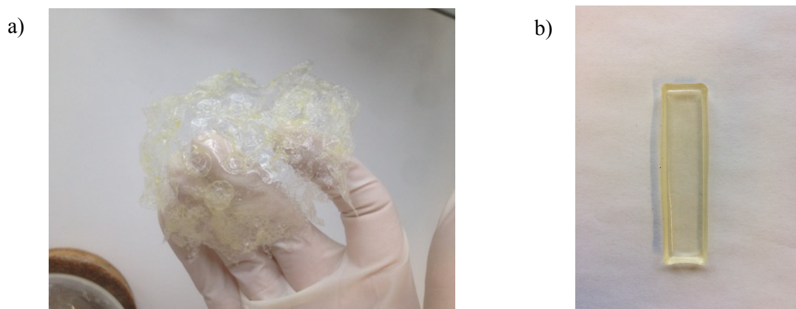
Figure 53 – a) Image of the product from the organotin-catalysed chain-extension/ cross-linking of polybutadiene with hexamethylene-1,6-diisocyanate (HDI); b) image of the same material after moulding.
