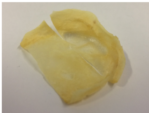
Figure 76 – Image of DOUBLE DYNAMIC recycled after neutralisation and evaporation of DOUBLE DYNAMIC from a THF solution
