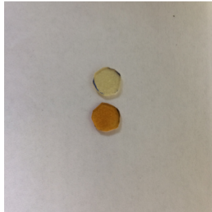
Figure 79 – Two pieces of DOUBLE DYNAMIC : above is a pristine sample; below after heating at 130 °C for 1 hour
