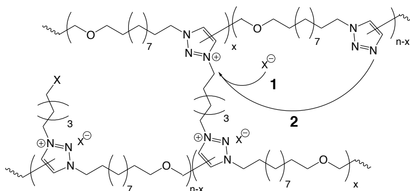
Scheme 14 –Transalkylation of triazonium salts via 1) nucleophilic attack of a halide counterion, or 2) concerted exchange.
