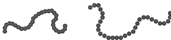
Figure 19 – Cartoon representing the difference between classical covalent polymers (left) and supramolecular polymers (right). 142
